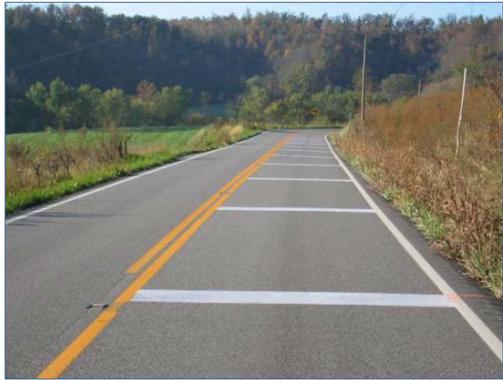
Figure 15. Equally-spaced transverse lines (Vest et al. 2005)
