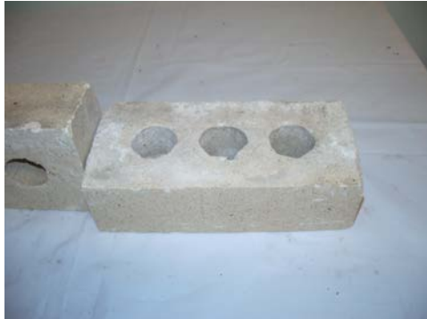
Figure 17. Sample 16: Residential Brick from Building Demolition.
