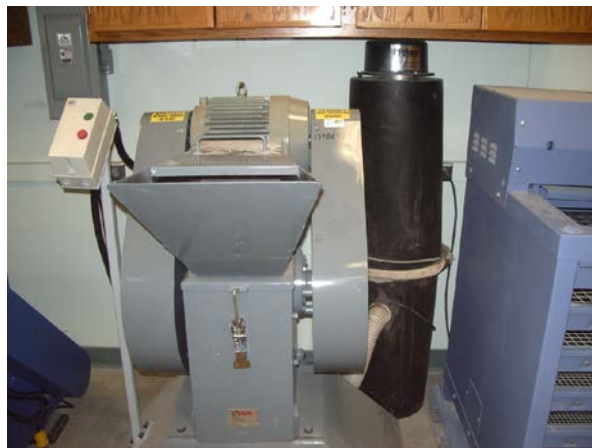
Figure 18. Jaw Crusher and Screen used to Crush Brick and Separate Sizes.
