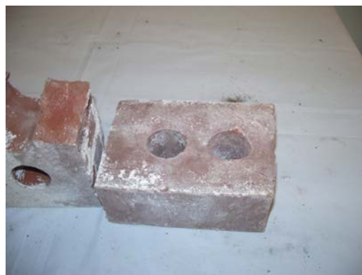
Figure 14: Sample 13: Residential Brick from Dorm Demolition.
