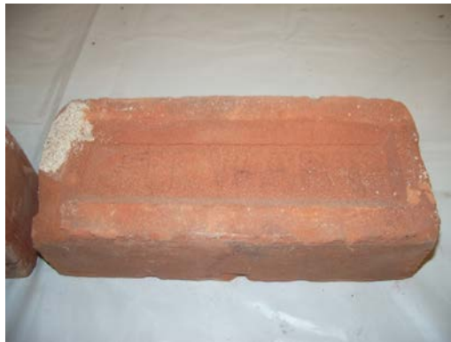
Figure 15. Sample 14: Refractory Brick from Cold Storage Building.
