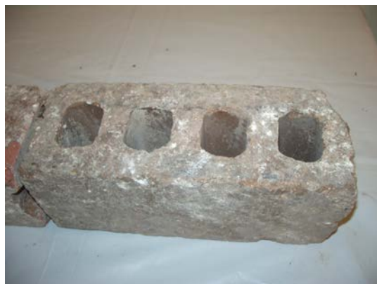
Figure 10. Sample 9: Commercial Brick from Stockpile.
