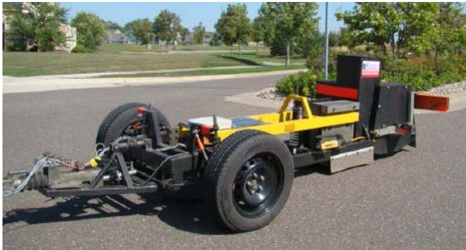
Figure 4-1. Rolling resistance test trailer. (Source: MnDOT [6]. Reprinted with permission.)
