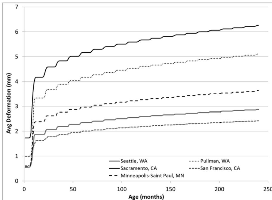
**Figure 4-21: TPF-5(149) procedure for rutting, sensitivity to climate.**
