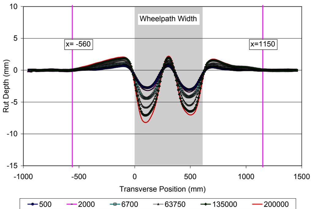
**Figure 4-15: Evolution of Section 609HB rutting profile.**
