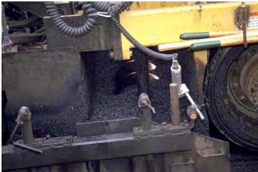
**Figure 5-9: HMA head in auger (Mahoney, Pavement interactive.com).**
