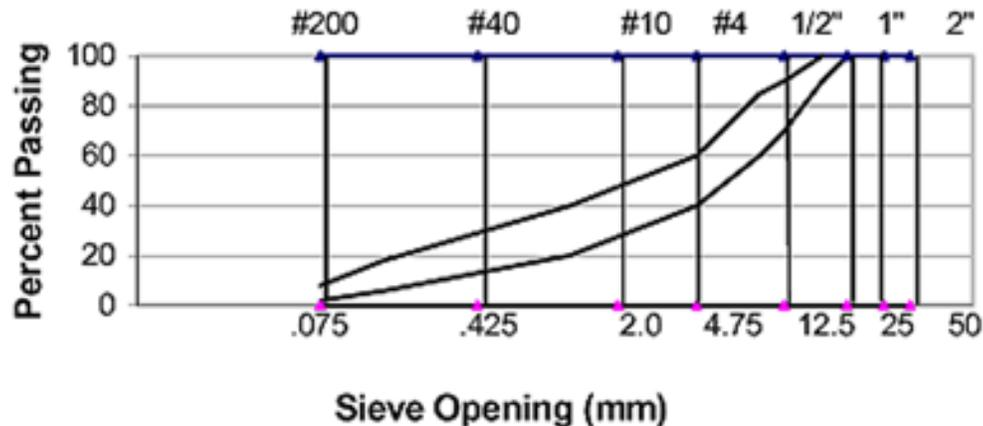
**Figure 5-5: Recommended aggregate gradation for RCC (from ACI 1995).**
