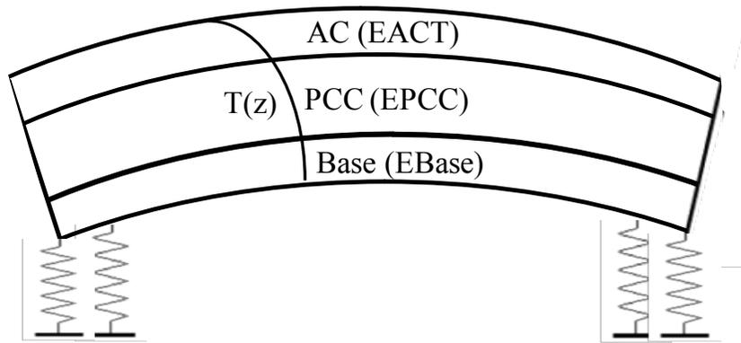
**Figure 3-29: System 1 under positive temperature gradient  $T(z)$  only.**
