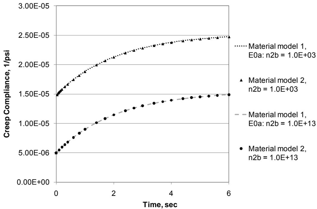
**Figure 3-23: Creep compliance for material models 1 and 2.**
