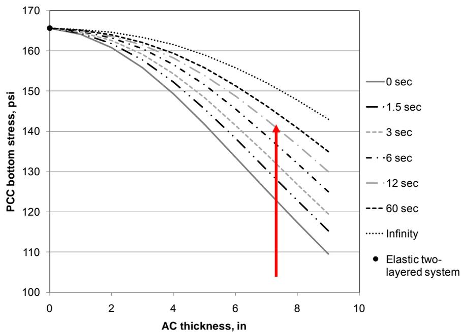
**Figure 3-26: PCC bottom stresses versus AC thickness.**
