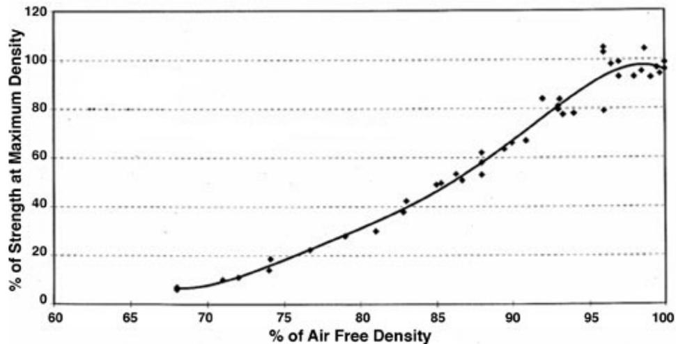
**Figure 5-7: Relation between compaction (measured as % air free density) and strength (from Schrader, 1992).**
