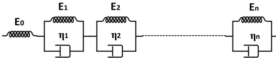
**Figure 3-9: Schematic of generalized  $N$ -term Kelvin-Voigt model.**
