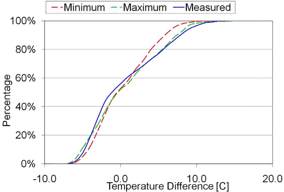
**Figure 2-26: Measured versus modeled cumulative frequency distribution for thermal gradient through JPCP pavement in July with  $k = 0.94$  BTU / hr-ft-°F.**
