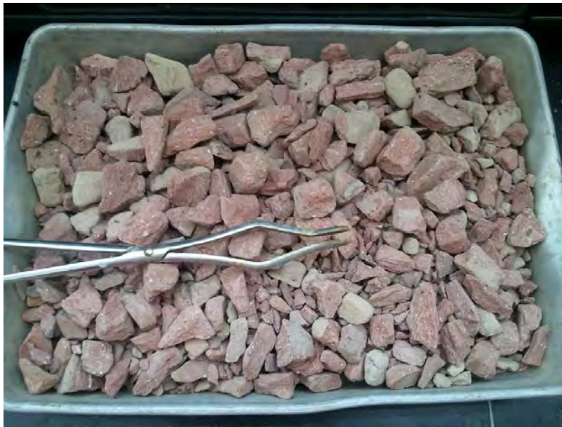
Figure 9.14 Crushing Brick and Final Product
