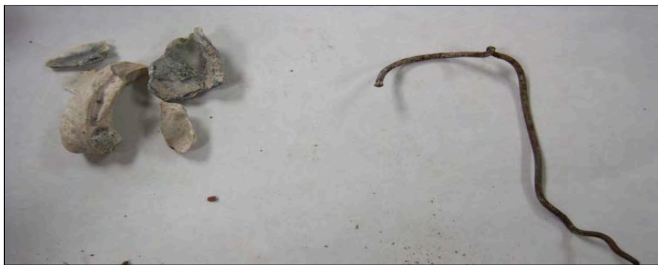
Figure 9.6 Deleterious Material Found in RCA: Sea Shells and Steel
