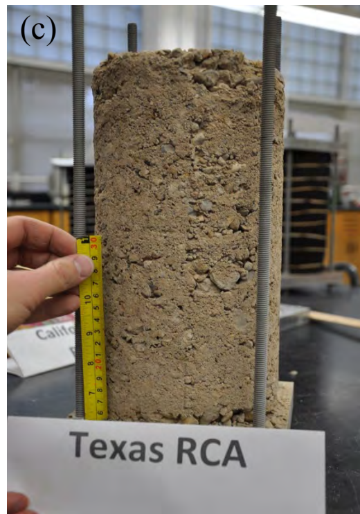
Figure 5.44 TX RCA after Wet/Dry Cycles: (a) 5 Cycles; (b) 10 Cycles; (c) 30 Cycles
