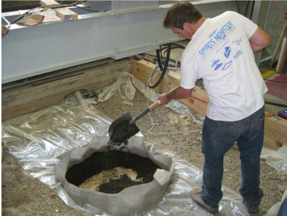
Figure A.2. Placement of RPM within Abbreviated Test Pit Area
