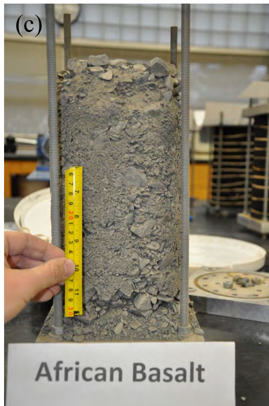
Figure 5.42 African Basalt after Wet/Dry Cycles: (a) 5 Cycles; (b) 10 Cycles; (c) 30 Cycles
