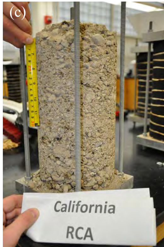
Figure 5.43 CA RCA after Wet/Dry Cycles: (a) 5 Cycles; (b) 10 Cycles; (c) 30 Cycles
