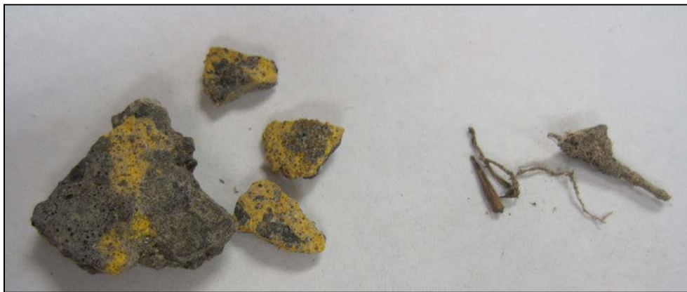
Figure 9.8 Deleterious Materials Found in RAP: Pavement Markings and Wood Chips
