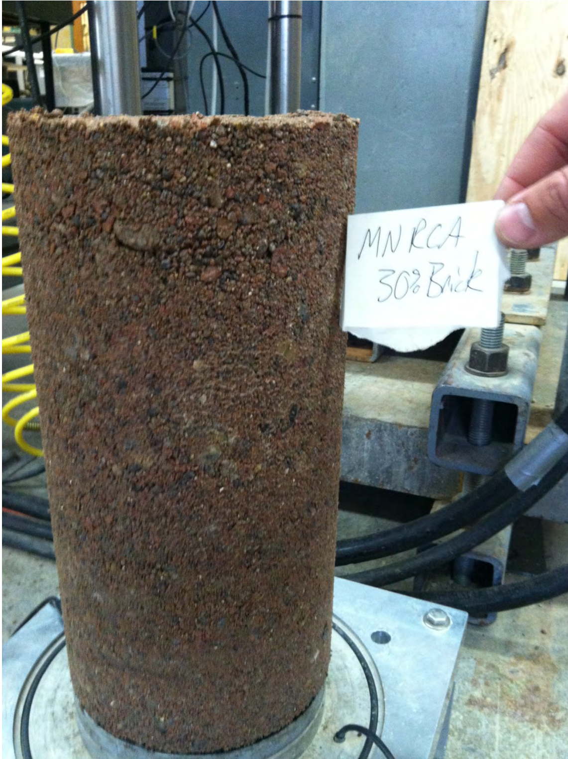
Figure 9.19 30% RCB with MN RCA compacted for Resilient Modulus Test
