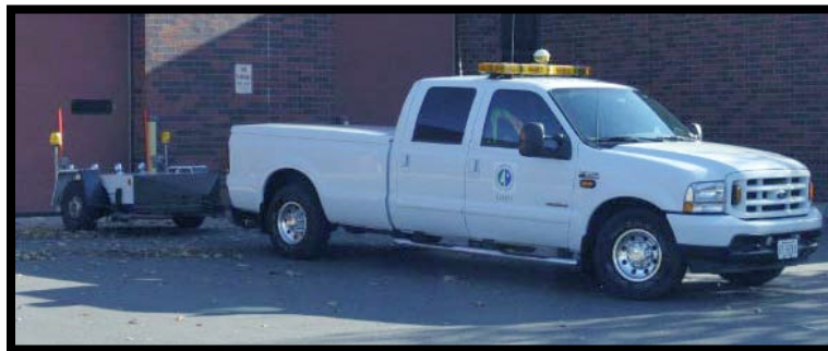
Figure 34: KJ Law Friction Trailer and Truck
