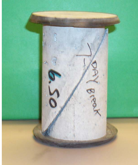
Figure 23: Slant Shear Specimen
