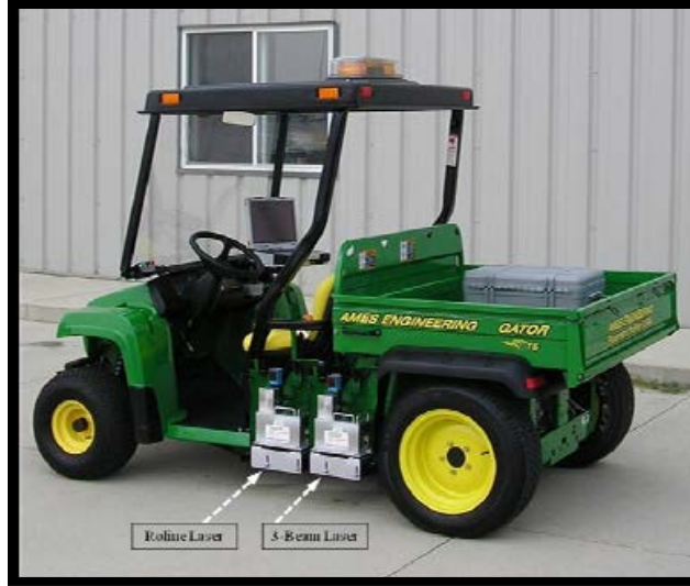
Figure 39: Lightweight Inertial Surface Analyzer
