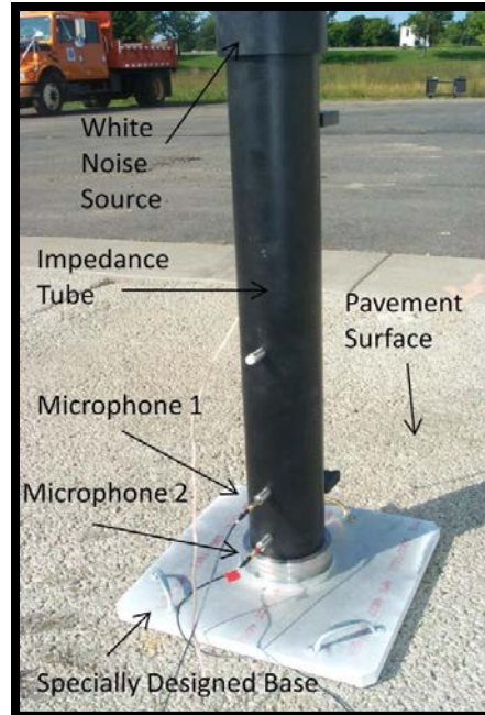
Figure 30: Sound Absorption Impedance Tube
