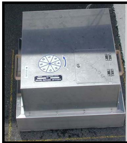
Figure 36: Circular Track Meter
