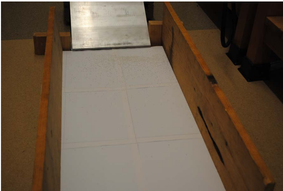
Figure 3. Bounce test apparatus showing aluminum plate (0 °F at start of test) inclined at 30° above horizontal, twin lines of capture paper, and side boards. Not shown is vial formerly containing 30.0 g of deicer (rock salt, passing #10 sieve, retained on #20 sieve) at 3 feet above floor (paper) level. Note spray pattern of deicer on paper.
