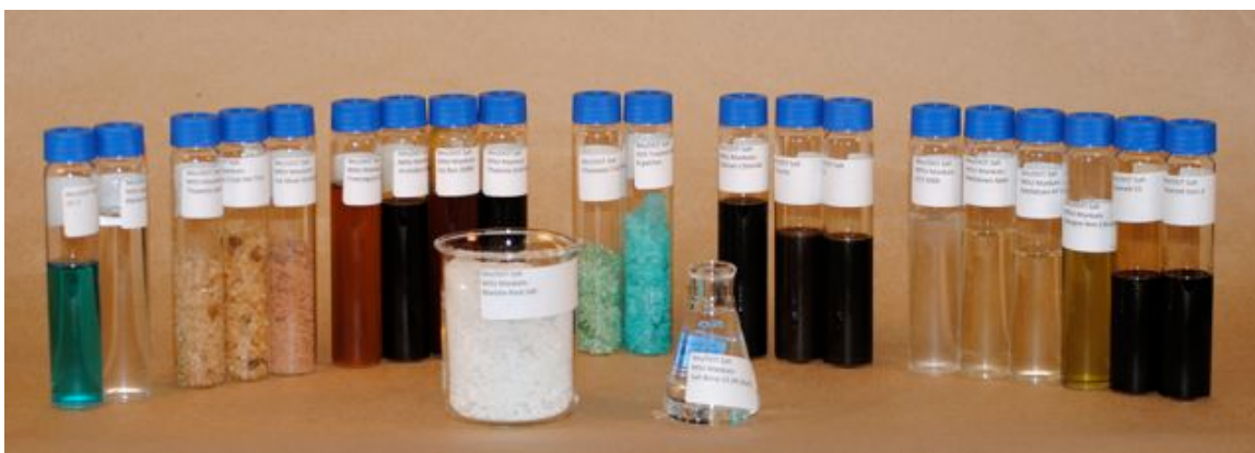
Figure 1. Deicers evaluated in this study, generally grouped as: (in center front) blanche rock salt (beaker), salt brine (flask), (from left) acetates (two vials), treated rock salts (three vials), magnesium chlorides (four vials), dyed magnesium chlorides (two vials), calcium chlorides (three vials), and carbohydrate/agricultural byproducts (six vials).
