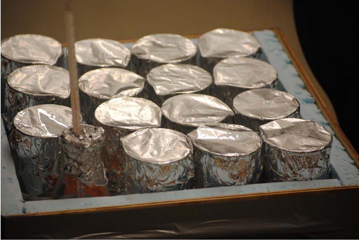
Figure 2. Ice specimens prepared for study in beakers within a thermal stabilization unit.
