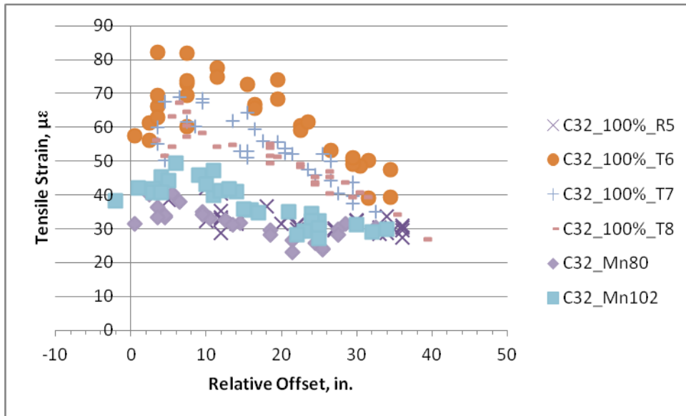
Figure 6.20. Cell 32 pavement strain responses during fall 2009 field testing at 100% load level
