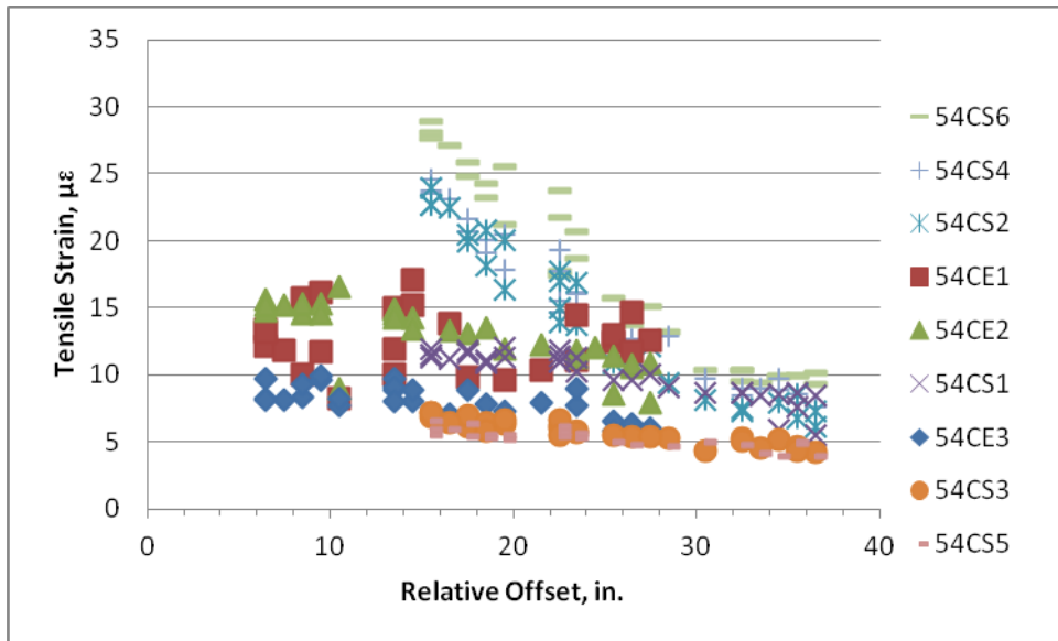
Figure 6.15. Pavement strains from all 9 sensors produced by Mn80 on cell 54
