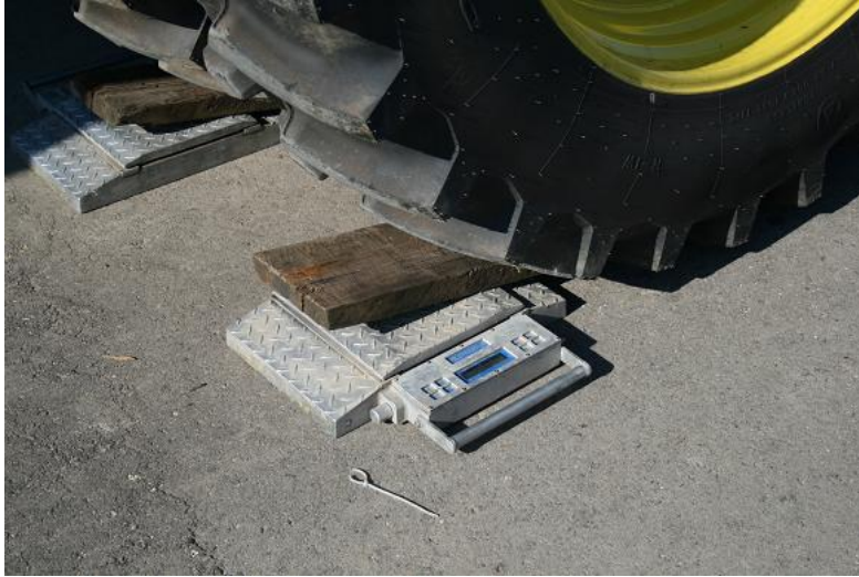
Figure 3.16. Weighing vehicles using portable scales
