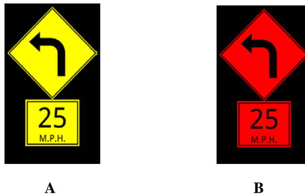
Figure 2.3. Examples of the A) advance curve speed notification and B) curve speed warning.
