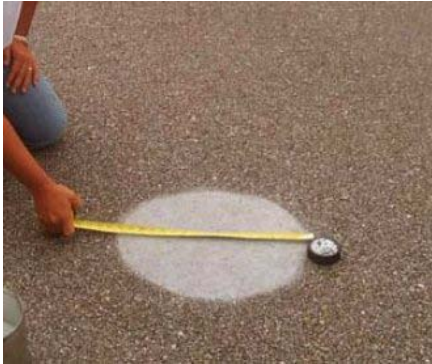
Figure 2.7: Procedure for Sand Patch Method
