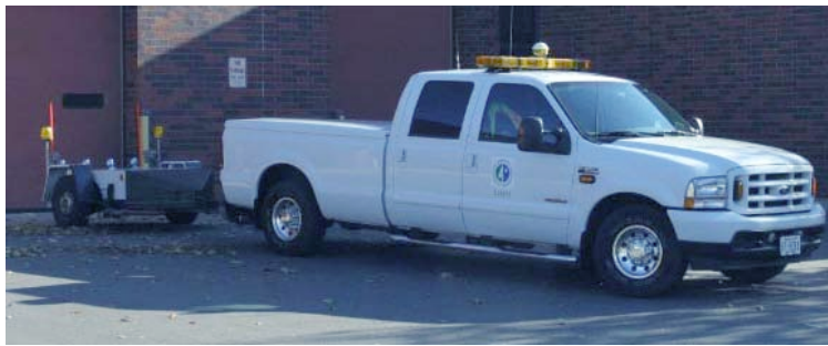
Figure 2.4: Locked-Wheel Skid Trailer and Truck
