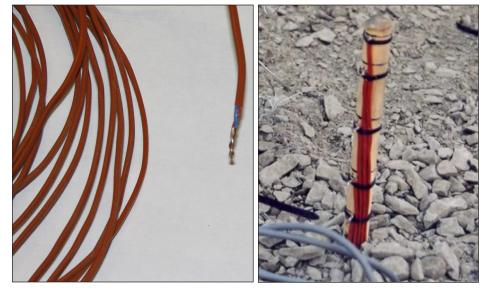
A thermocouple sensor (left) is typically mounted on a vertical tree (right) spanning surface and subsurface pavement layers, allowing temperature measurements at various depths. These vertical profiles are critical to fully relating pavement performance to temperature.
