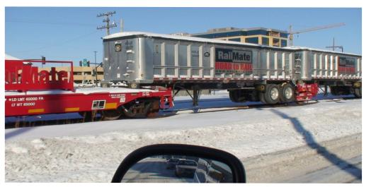
The taconite used in this study was delivered via specialized trailers that can travel by rail or semitractor, demonstrating a promising option for future long-distance hauling of taconite aggregates to road construction projects where local aggregates are scarce.
