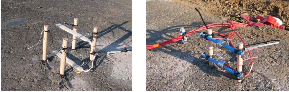
Figure 2.3. Dynamic Strain Sensors [Left] and Environmental Strain Sensors [Right]
