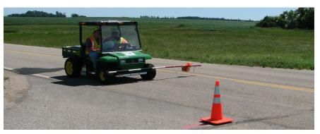
IRI algorithms for calculating ride quality from pavement profiles use data from inertial profilers, which use laser sensors to take precise measurements per inch of pavement.
