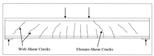
Excessive shear—the net force on a girder perpendicular to its length resulting from the pilings holding up the ends and the supported weight pushing down across the span—can crack the concrete of a girder, possibly compromising its strength.
