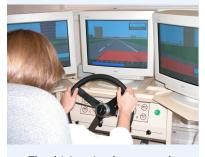
The driving simulator console had three 17-inch CRTs, a steering wheel and pedals, and an automobile seat. Speakers behind the CRTs simulated engine noise.
