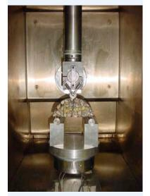
In the Semi-Circular Bend test, a load is applied to a halved asphalt mixture core sample while gages are used to record resulting cracks.
