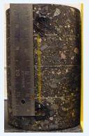
Counties provided 6-inch-diameter wear and nonwear course core samples for the evaluation of dynamic modulus and other properties.
