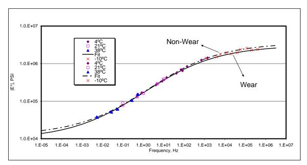
Figure 24 – |E\*| master curve for Olmsted CR 112 wear and non-wear course specimens; 58-34 with no RAP.
