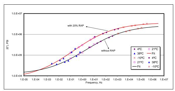
Figure 25 – |E\*| master curve for Olmsted CR 112 full depth cores; 58-34.
