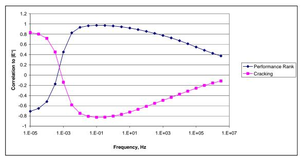
Figure 31 – Relationship of field performance and |E\*| master curves.
