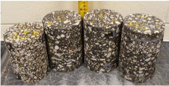
Figure 15 – |E\*| specimen set from Olmsted CR 112 cores.
