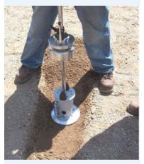
LWDs determine stiffness by measuring the deflection of the ground induced by a dropped weight.
