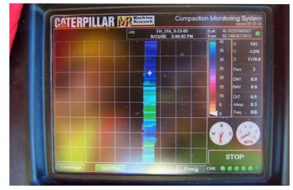
IC rollers are equipped with a Global Positioning System to map the location, time and force of compaction. This data is stored for future use in forensic analysis, long-term pavement management and mechanistic-empirical pavement design.
