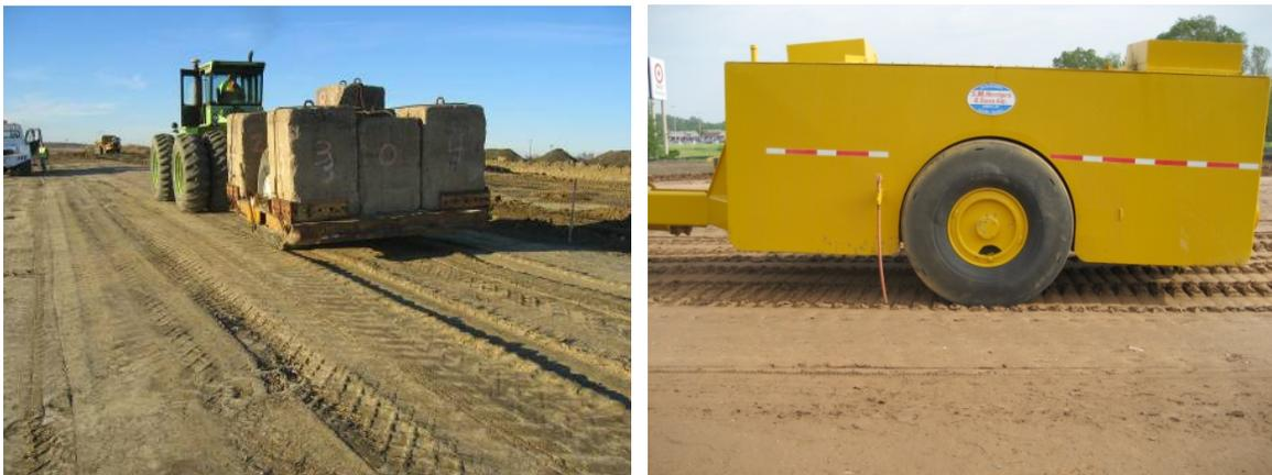
Figure 4.1. Towed pneumatic dual-wheel test rollers with 650 kPa contact tire pressure used on TH14 (left), TH60 (left) and TH36 (right) project
