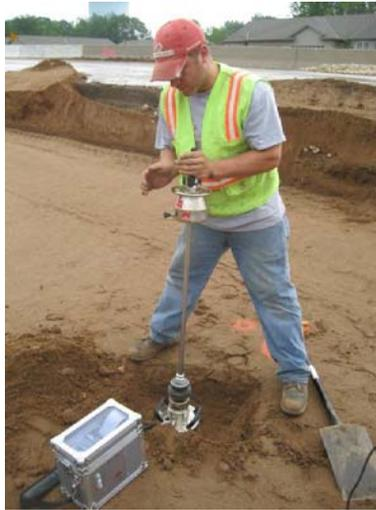
Figure 5.19. LWD test in an excavation by removing loose material at the surface to a depth of about 100 to 200 mm for cohesionless materials
