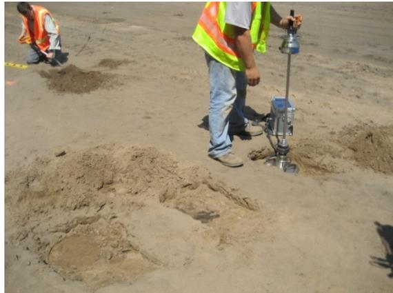
Figure 3.32. LWD testing performed by excavating loose material at the surface to a depth of about 0.15 m
