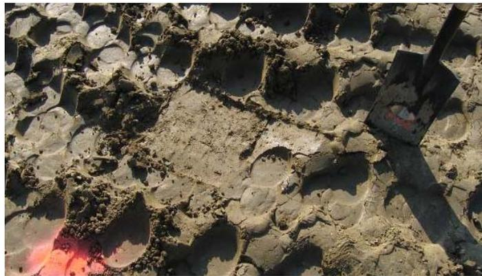
Figure 5.20. Level surface at the bottom of the padfoot impression for non-granular materials
