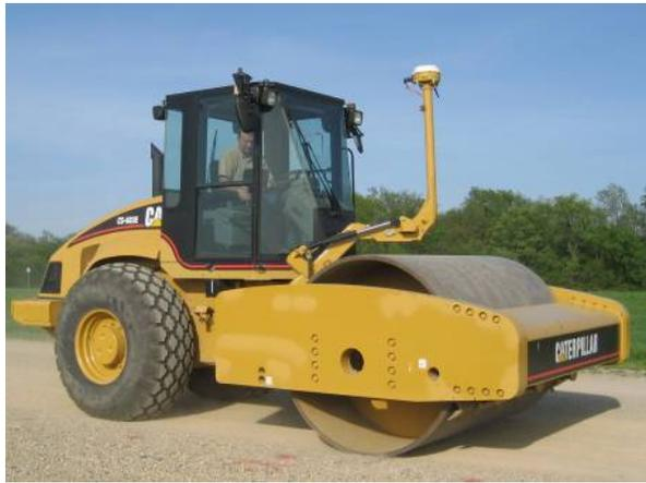
Figure 2.1. 12-ton CS-563 smooth drum (left) and 19-ton CS-683 smooth drum rollers equipped with CMV/RMV systems and GPS
