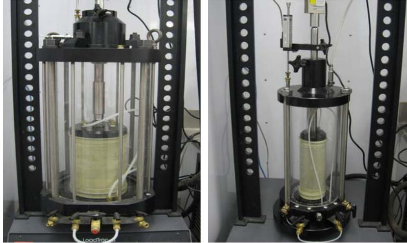
Figure 5.37. Resilient modulus testing on 1:1 and 2:1 gyratory compacted specimens
