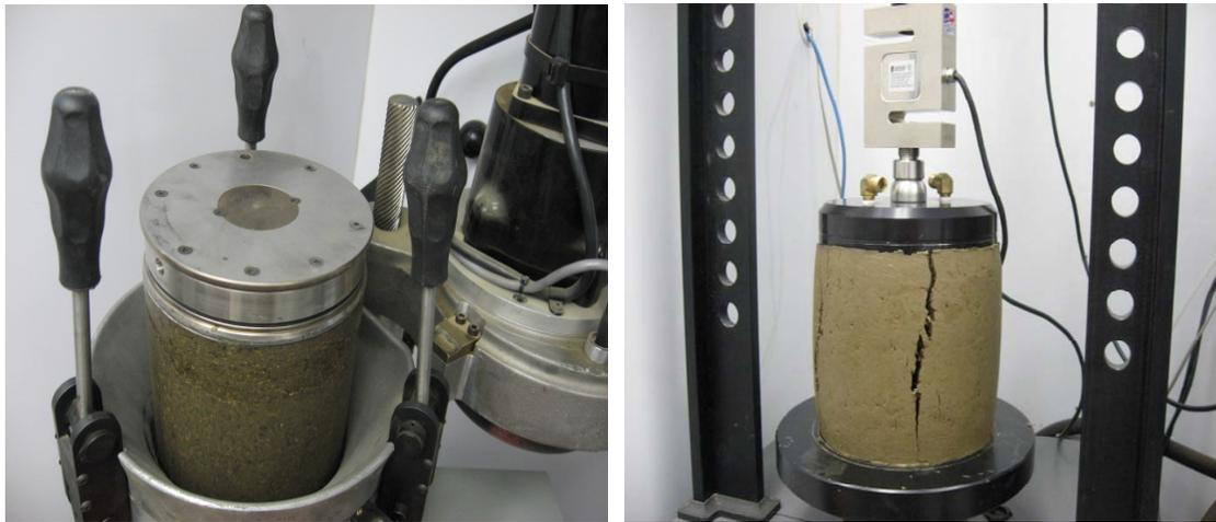
Figure 5.36. PDA (left) and unconfined compression test (right) on gyratory compacted specimen
