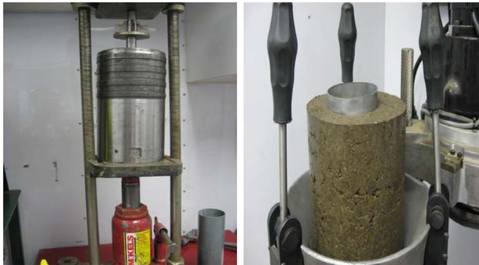
Figure 5.38. Procedure for inserting Shelby tube into gyratory compacted specimen to generate 2:1 height to diameter ratio specimens
