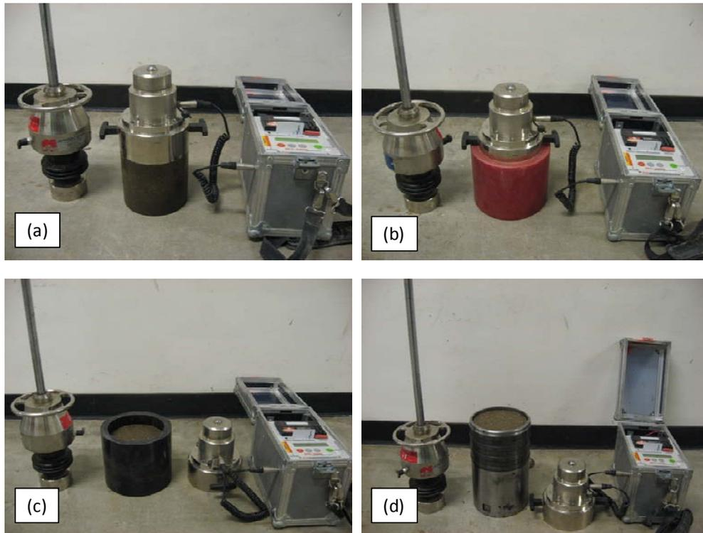
Figure 5.34. LWD testing with four different boundary conditions: (a) no boundary, (b) soft polyurethane (Durometer = 20A), (c) stiff polyurethane (Durometer = 50A), and (d) rigid gyratory compaction mold
