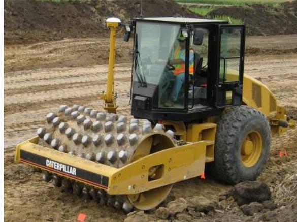
Figure 2.2. 12-ton CP-563 padfoot roller equipped with MDP\* system and GPS
