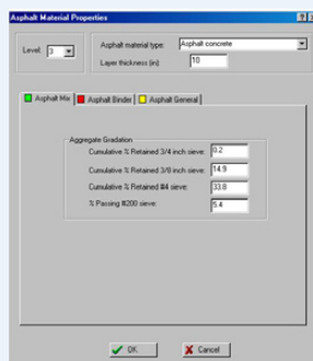
An MEPDG software input screen for specifying asphalt layer thickness in inches.
