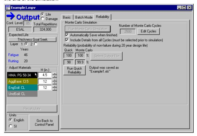
Quick Reliability uses equations derived from running a range of full Monte Carlo simulations to estimate the Monte Carlo reliability for a given structure. This is a time-saving feature that allows quick adjustments in the structure. Once the desired quick reliability value is reached a full Monte Carlo reliability should be run for verification.
