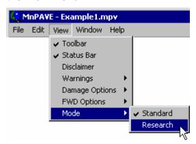
In Research Mode there are more features and more flexibility in entering data. However, there is one important difference in the way hot-mix asphalt (HMA) modulus is determined. In Standard Mode, all asphalt binders have the same properties as PG 58-28 for the following reasons:
