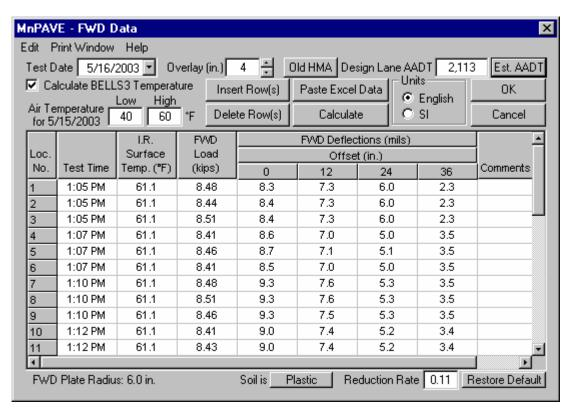
Pavement temperature can be entered by two methods. If the pavement temperature is known, uncheck the Calculate BELLS3 Temperature checkbox and enter the known pavement temperature values in column 2. If the pavement temperature is not known, it can be estimated using the BELLS 3 method. Enter the previous day's high and low air temperatures in the appropriate boxes and the infrared surface temperatures in column
