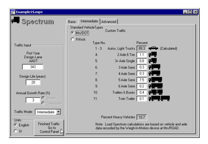
Vehicle types are quantified in pavement design procedures to more accurately define the loads on the pavement. Vehicle type data can be obtained from manual counts or from automatic vehicle classification systems. The Mn/DOT classification system differs somewhat from the FHWA system. Data in FHWA format can be entered and MnPAVE will convert it into Mn/DOT format. Vehicle-specific axle weight distributions are used to convert vehicle type data into a load spectrum for pavement simulations.
