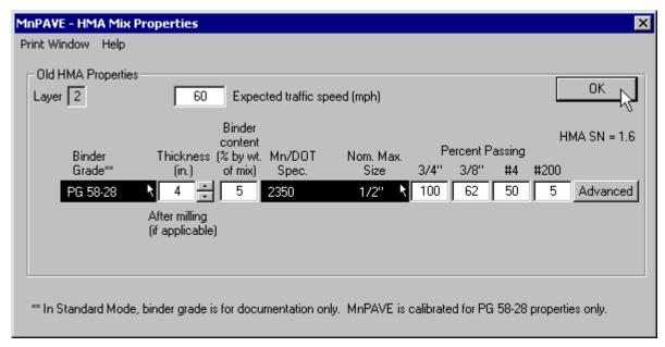
If the HMA Mix Properties window did not open, click on the gray Old HMA subtype bar. Select the binder grade of the old HMA and any other mix properties that are known and click OK.
