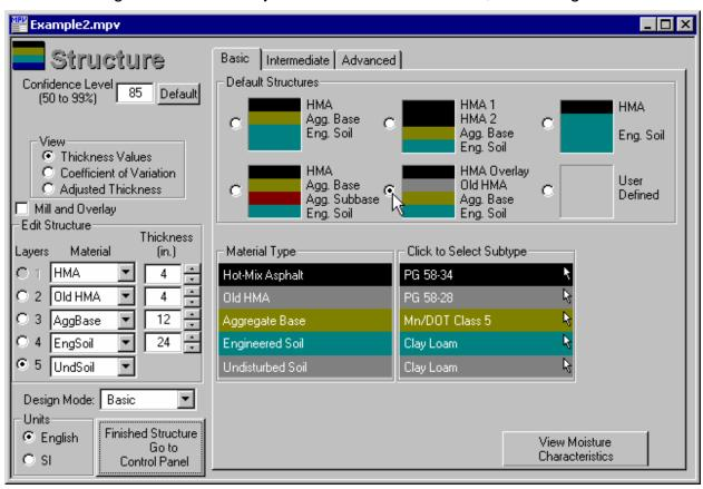
Select the default overlay structure. If the old HMA properties for this layer have not yet been defined, the HMA Mix Properties window will open up.
