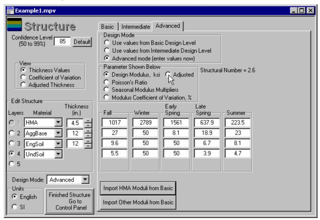
The design mode is displayed above the "Finished" button to confirm that the correct mode is selected. Any editing that is done in the Basic, Intermediate, or Advanced windows will change the mode. If any editing causes the wrong mode to be selected, this can be corrected prior to clicking on the "Finished" button.
