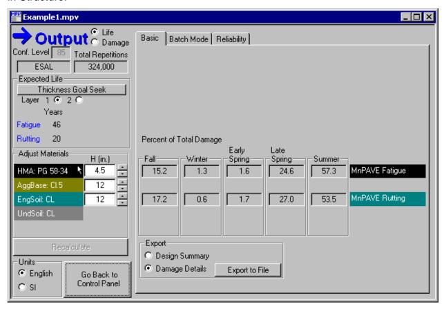
When Thickness Goal Seek is done for non-HMA layers, the HMA layer will be adjusted for fatigue first (if necessary), and then the selected layer will be adjusted. This is because adjusting underlying layers has a relatively small effect on fatigue life and may result in a large number of cycles and very thick layers.
