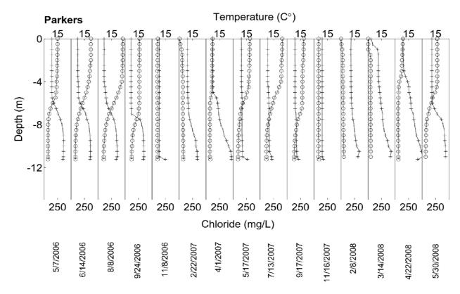
Figure 4.10 Chloride and temperature profiles in Parkers Lake.
