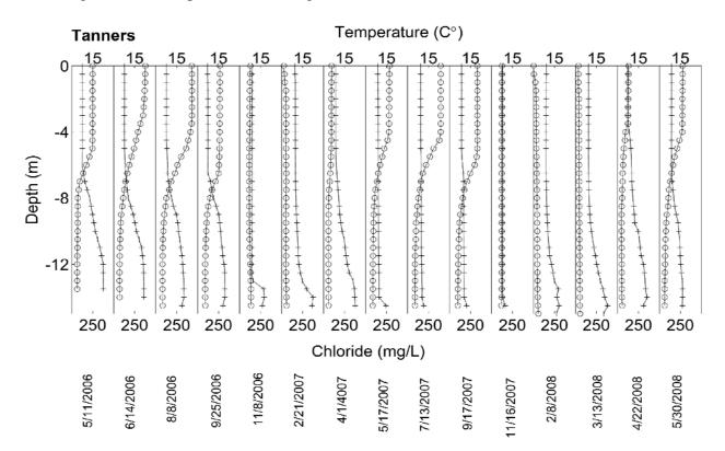
Figure 4.9 Chloride and temperature profiles in Tanners Lake.
