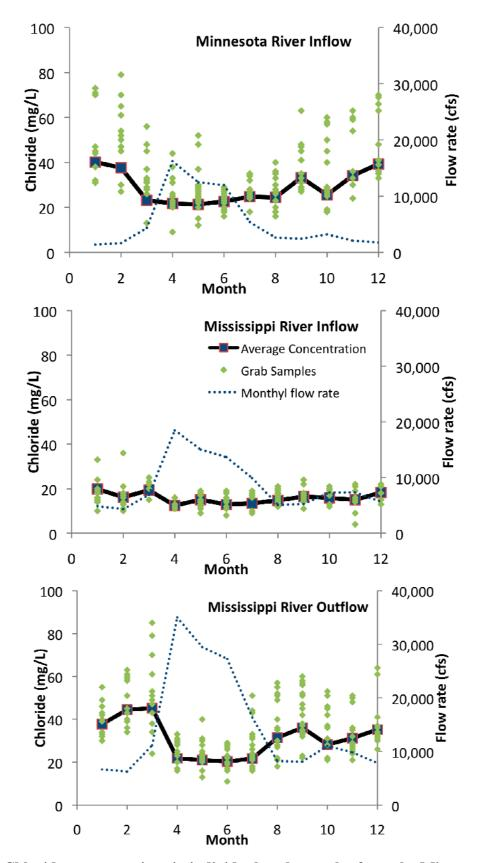
Figure 3.3 Chloride concentrations in individual grab samples from the Minnesota and Mississippi Rivers. Flow-weighted average monthly values for concentrations and flow rates are plotted as solid and dotted lines, respectively. All values are from measurements taken between the years 2000 and 2007.
