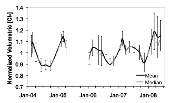
Figure 4.7 Seasonal salinity (CI<sup>°</sup>) cycles illustrated by normalized (volume-weighted) average chloride concentrations. Averages are for all lakes in each time period. Bars represent the standard deviation for the set of lakes. Reference for normalization is the (volume-weighted) average concentration for each lake during the sampling period.
