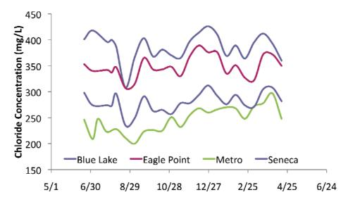
Figure 3.7 Chloride concentrations in WWTP effluents (June 2007-May 2008).
