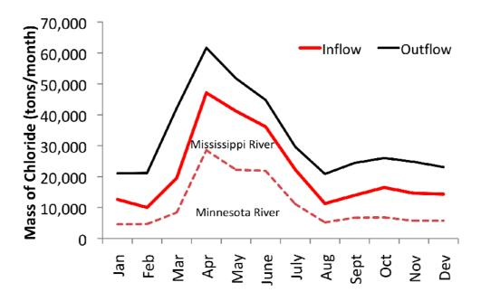
Figure 3.5 Mean monthly (2000-2007) chloride transport (tons/month) by the Minnesota and the Mississippi River into and out of the Metro watershed.
