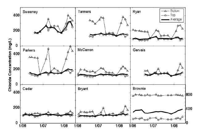
Figure 4.6 Chloride concentrations 0.5 m below the surface and 0.5 m above the bottom of 9 TCMA lakes, and average chloride concentrations in each lake sampled from Jan 2006 to May 2008.
