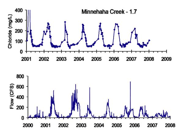
Figure 4.1 Chloride concentrations in Minnehaha Creek (1.7 miles from its outlet into the Mississippi River).
