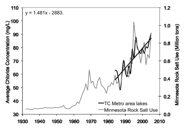
Figure 4.12 Comparison of lake chloride concentrations in 39 TCMA lakes and rock salt purchases by the state of Minnesota (Novotny et al. 2007).
