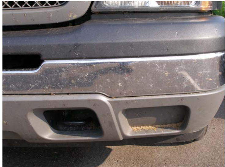
Figure 3-2. Seeds lodged in vehicle light reservoir
