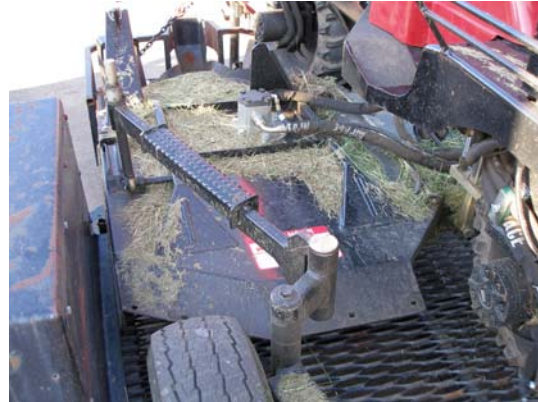
Figure 3-1. Mowing clippings completely covering mower decks
