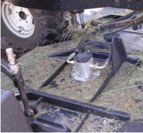
Figure 3-1. Mowing clippings completely covering mower decks
