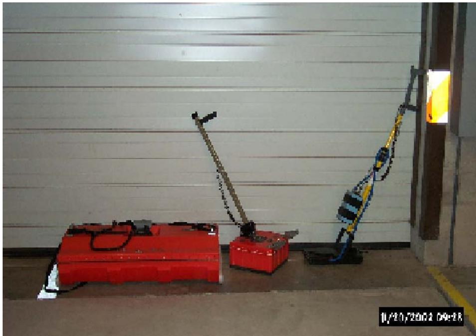
Figure 3.2 Ground Coupled GPR Antennas
