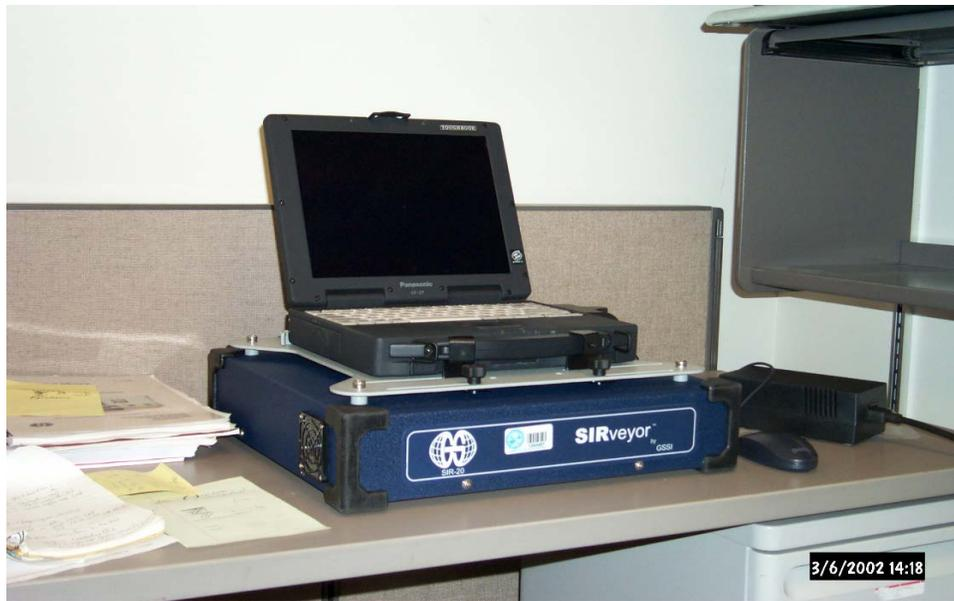
Figure 3.1 SIR-020 GPR Data Collection System
