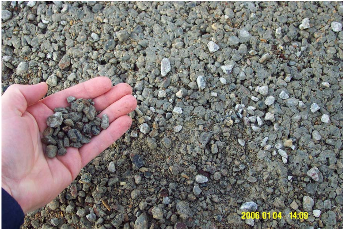
Figure C4. Mix #2, Surface Raveling, 01.04.06
