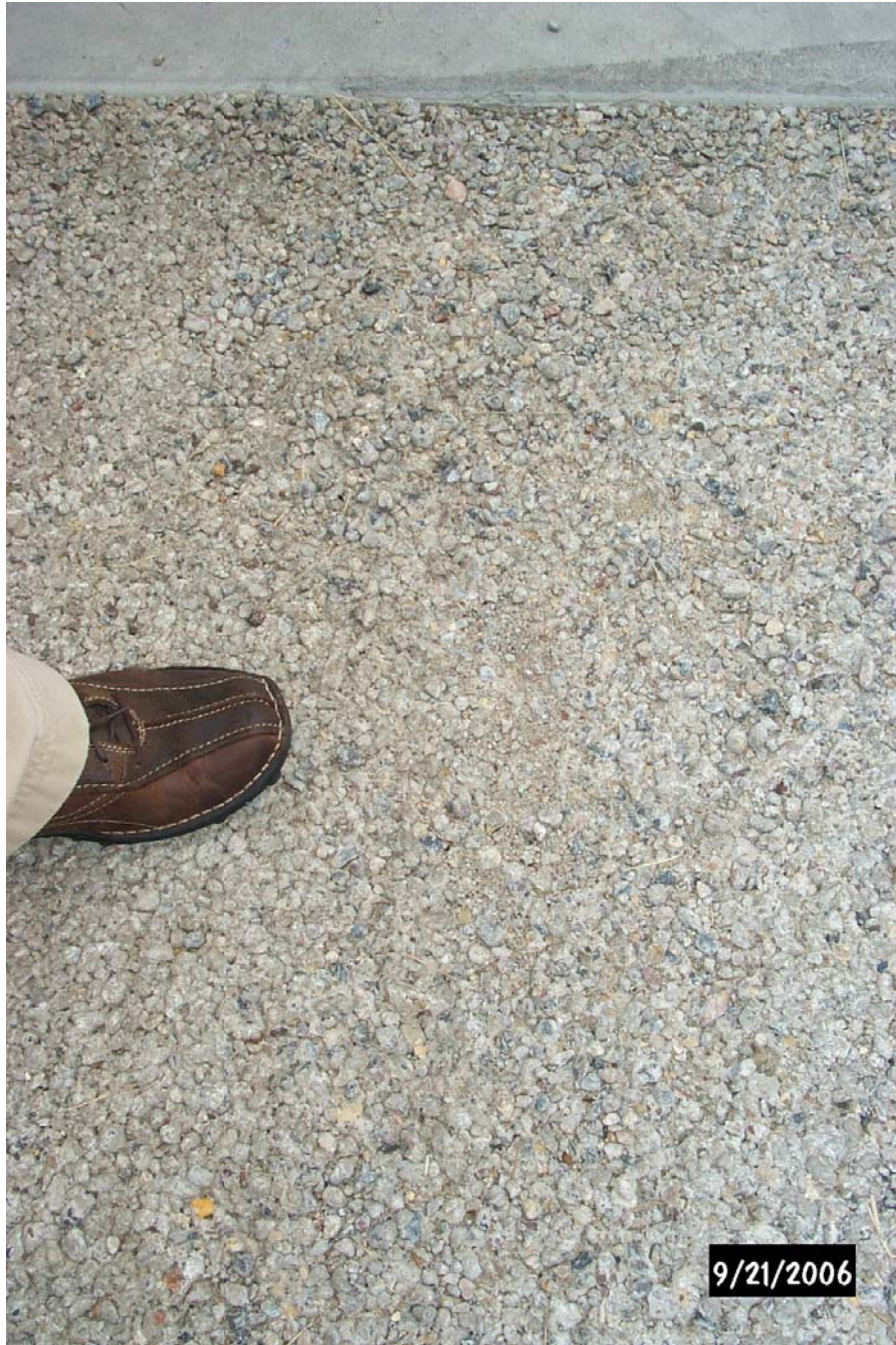
Figure C3. Mix #2 Surface Raveling, West Edge Cell 64, 9.21.06
