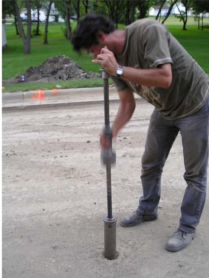
Fig. A7. Collecting a sample in a thin-wall tube using a drive-tube hammer.
