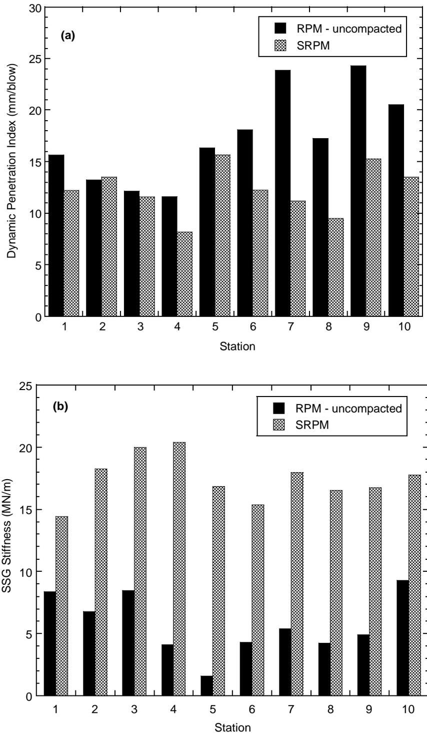
Fig. 10. Dynamic penetration index (DPI) and stiffness of uncompactd RPM and SRPM after compaction and 7 d of curing. DPI was measured with a DCP and stiffness was measured with a SSG.
