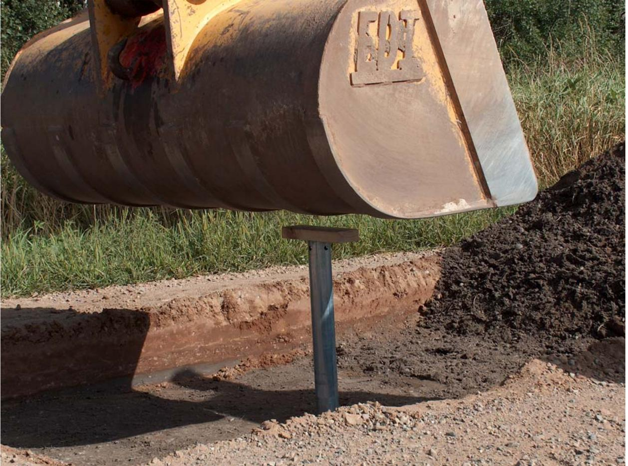
**Fig A5. Collecting a sample in a thin-wall tube**
