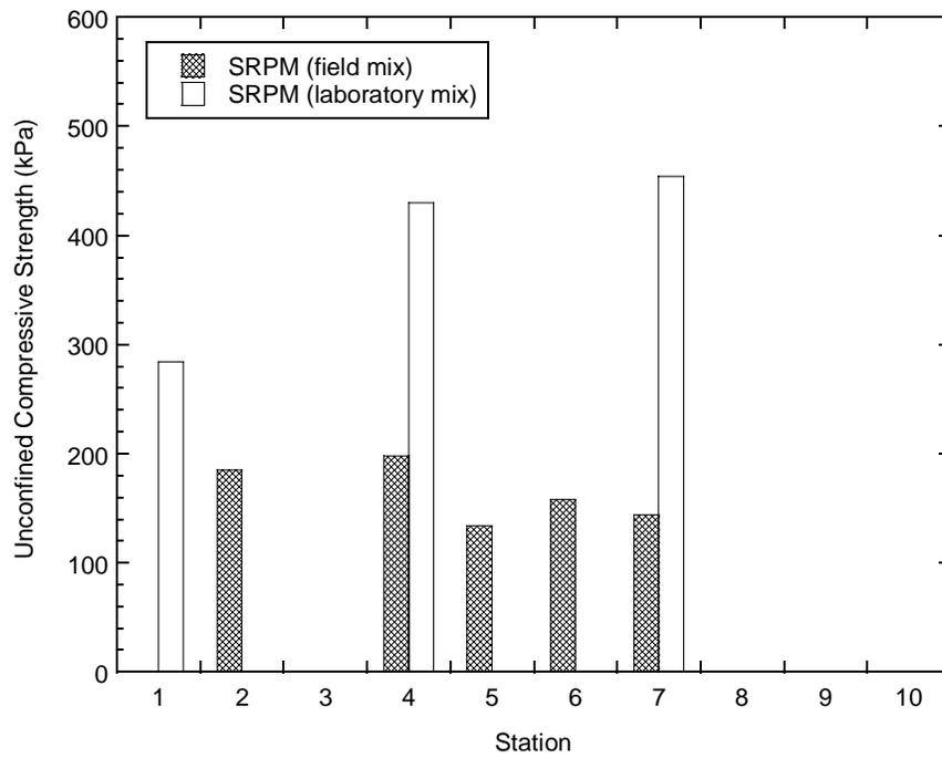
Fig. 9. Unconfined compressive strength ( $q_u$ ) of SRPM (laboratory-mix and field-mix) after 7 d of curing.
