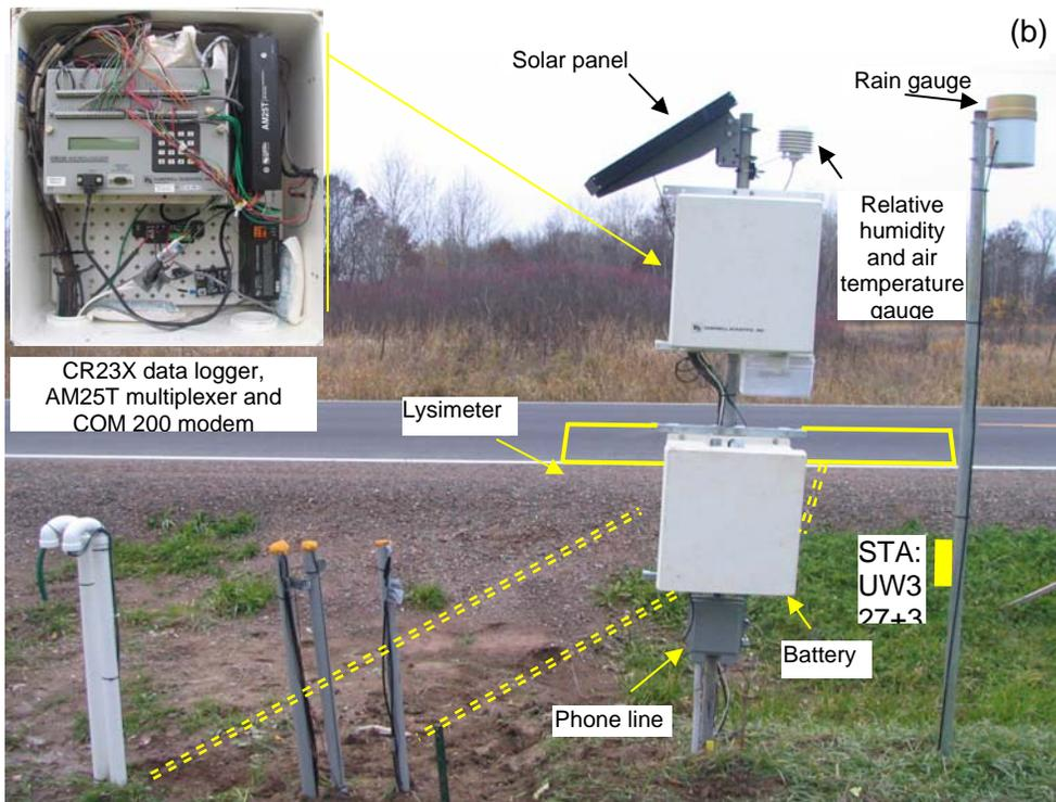
Fig. 8 (a) Layout (b) Photograph of completed field monitoring instrumentation system.
