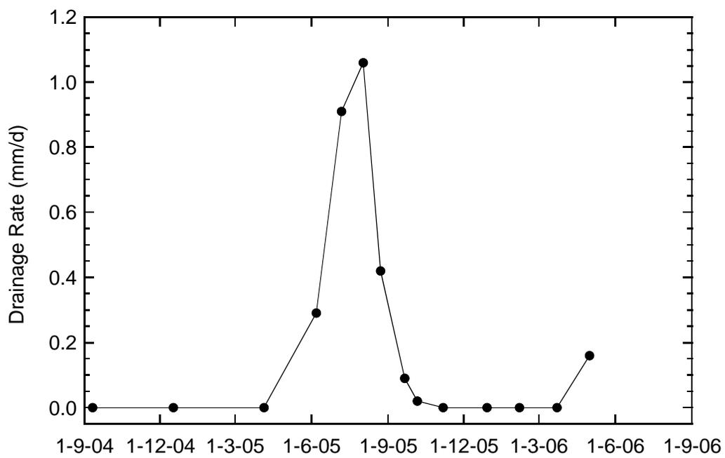
Fig. 4. Drainage from the pavement collected in the lysimeter. Base of lysimeter is located at the bottom of the SRPM layer.
