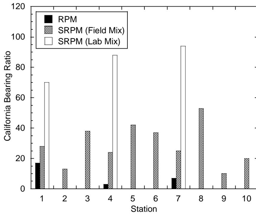
Fig. 7. California bearing ratio of RPM and SRPM (laboratory-mix and field-mix) after 7 d of curing.
