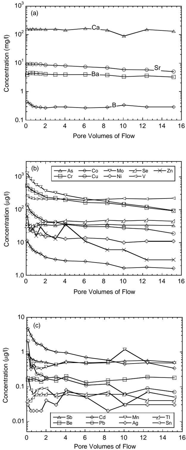
Fig. 18 Concentrations of trace elements in effluent from CLT on CH2 (Chisago Station 2): elements with peak concentrations (a) exceeding 1 mg/L, (b) elements with peak concentrations exceeding 10 µg/L, but less than 1 mg/L, and (c) elements with peak concentrations less than 10 µg/L.
