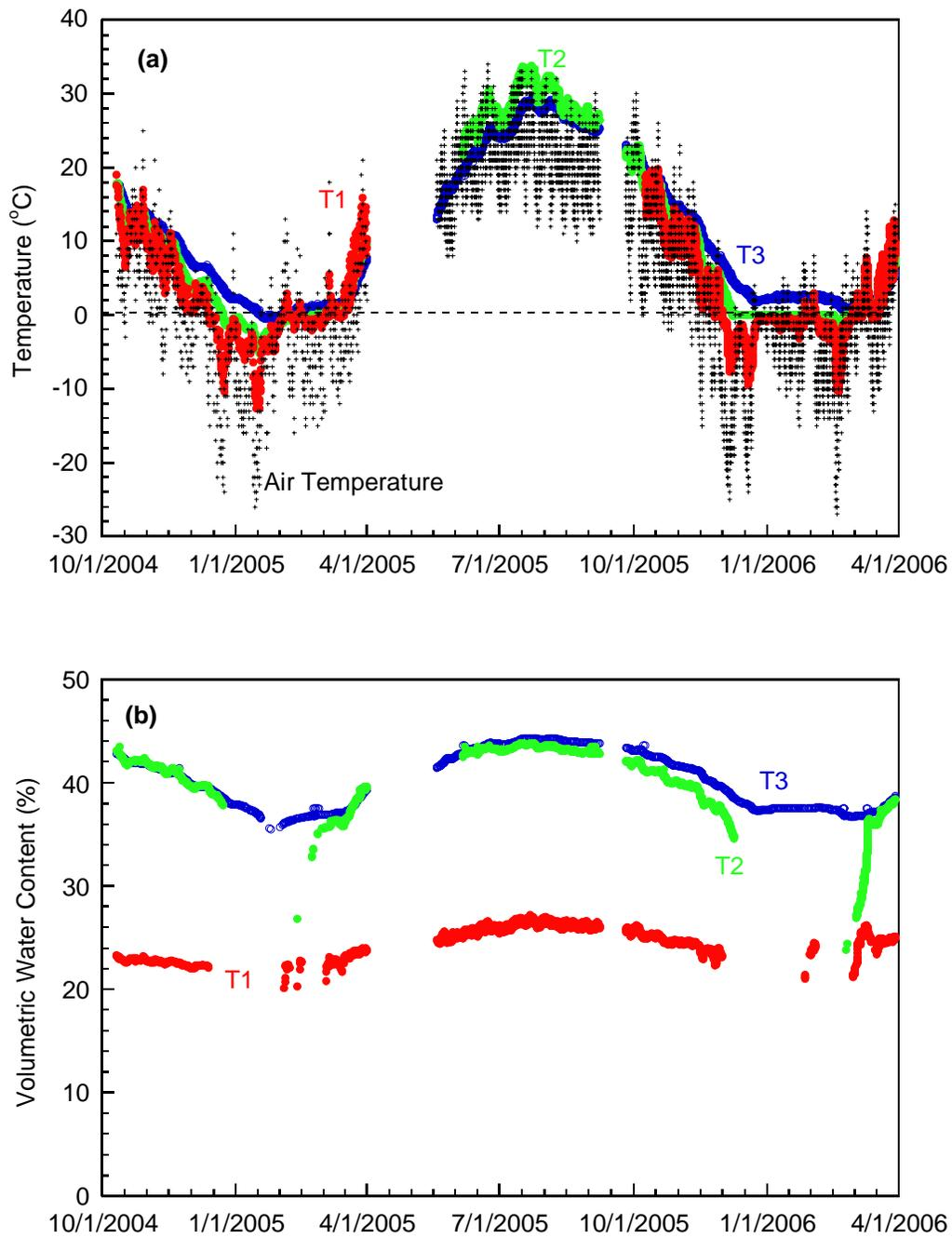
Fig. 3. Air and soil temperatures (a) and volumetric water content (b) of the SRPM and subgrade. Air temperature is shown in black. Soil temperature and water content measured at three depths: 150 mm bgs (mid-depth in SRPM) shown in red and designated as T1, 425 mm bgs (subgrade) shown in green and designated as T2, and 675 mm bgs (subgrade) shown in blue and designated as T3.
