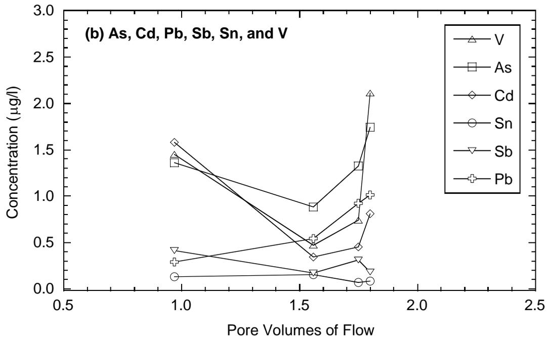
Fig. 5. Concentrations of trace elements in leachate collected in lysimeter: (a) elements with peak concentrations between 3 and 102  $\mu\text{g/L}$  and (b) elements with peak concentrations less than 2.5  $\mu\text{g/L}$ .
