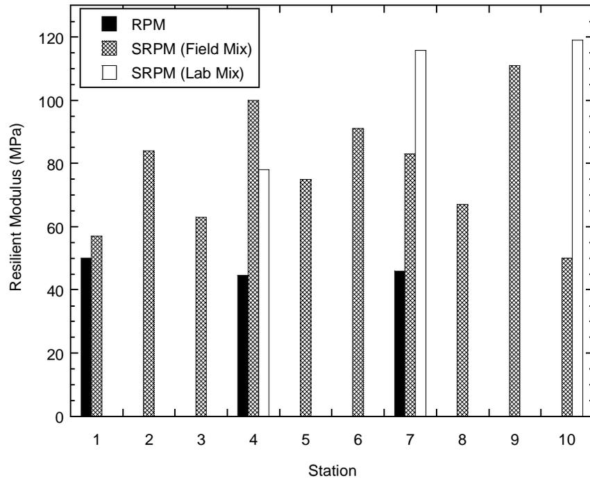
Fig. 8. Resilient modulus of RPM and SRPM (laboratory-mix and field-mix) after 14 d of curing.
