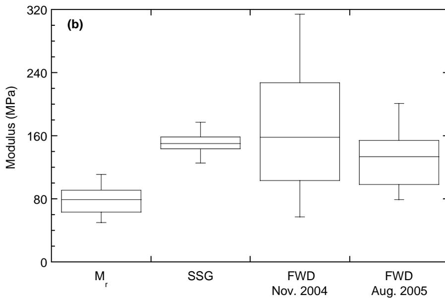
Fig. 12. Modulus of SRPM obtained by inverting FWD data, from SSG measurements, and from resilient modulus tests conducted in the laboratory: (a) modulus along the alignment and (b) box plots of each set of modulus measurements.
