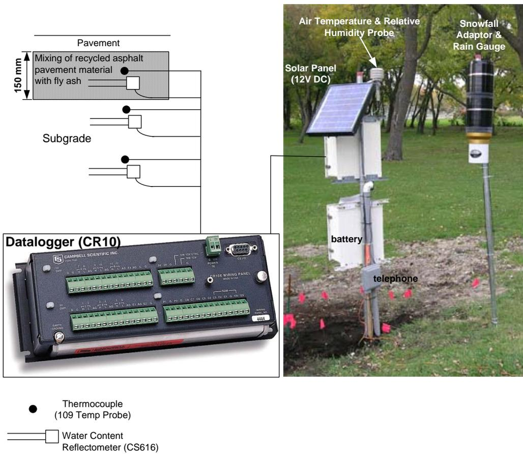
Fig. B4. Layout of field instrumentation.
