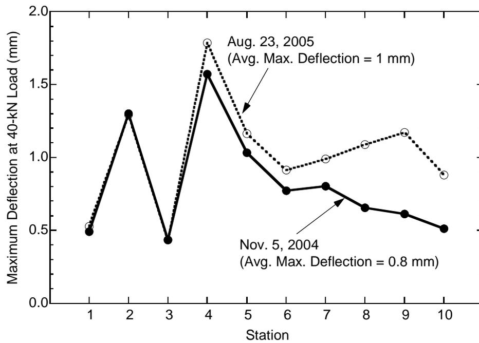
Fig. 11. Maximum deflection from the 40-kN drop for FWD tests conducted in November 2004 and August 2005.
