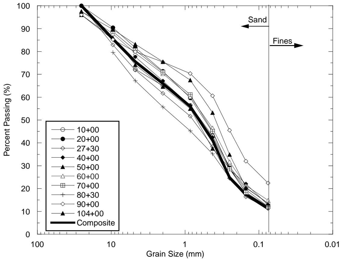
Fig. 4 Grain size distribution curves of RSG at sampling stations and composite of all stations.
