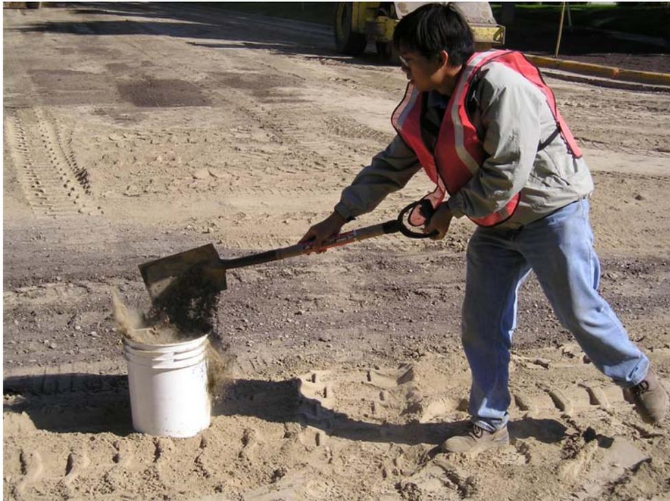
Fig. A6. Collecting a sample of fly ash for use in laboratory testing.
