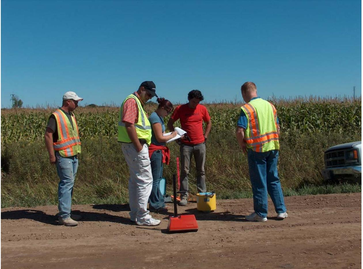
**Fig A11. Nuclear gauge and SSG tests on S-RSG.**
