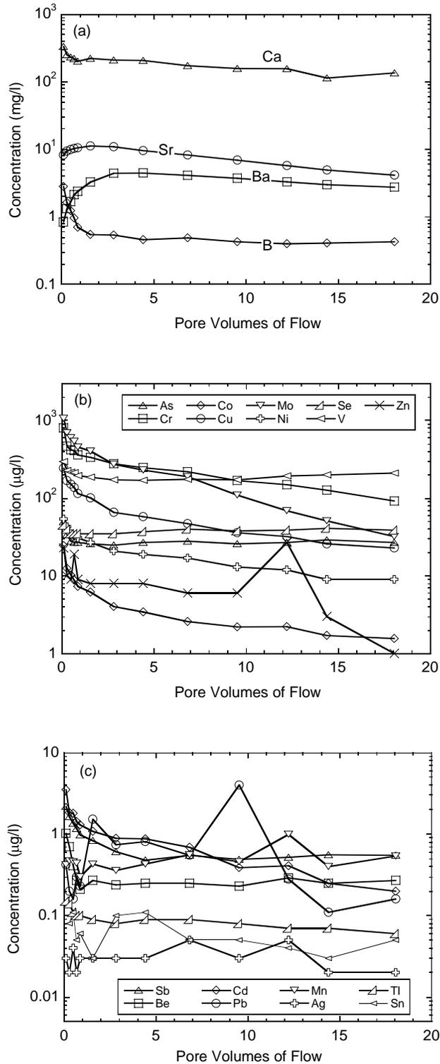
Fig. 19 Concentrations of trace elements in effluent from CLT on CH5 (Chisago Station 5): elements with peak concentrations (a) exceeding 1 mg/L, (b) exceeding 10 µg/L, but less than 1 mg/L, and (c) less than 10 µg/L.
