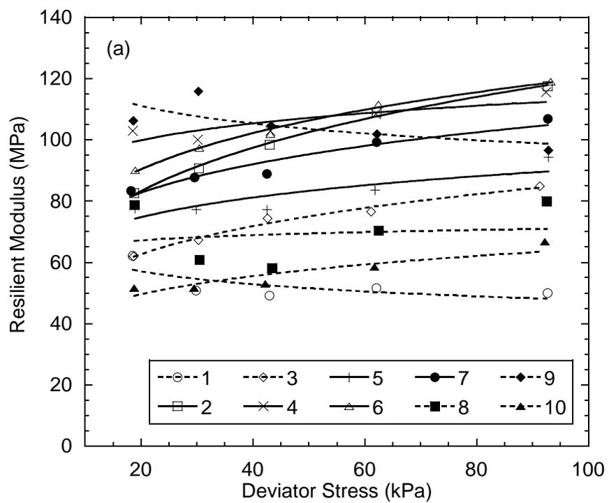
Fig. E1. Resilient modulus curves for SRPM.
