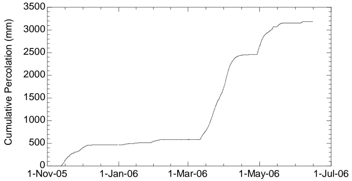
Fig. 16 Cumulative percolation into Lysimeter.
