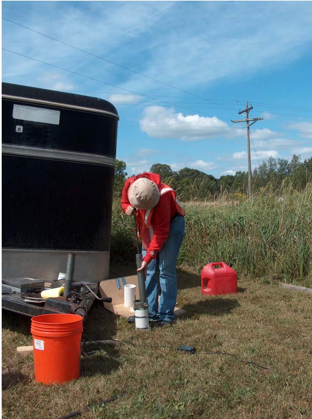
**Fig A13.  $M_r$  and CBR sample preparation of field mix soils collected with in 1-2 hour of blending process.**
