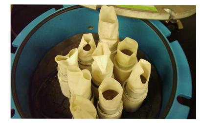
To bring soil specimens to a given level of soil suction, the specimens were placed in rubber sleeves and put in a pressure chamber.
