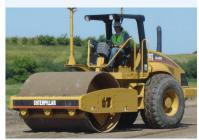
In Field Study 1, researchers used a Caterpillar CS-563 vibratory smooth drum roller to collect machine drive power and compaction meter value measurements.
