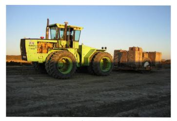
Test rolling on one project verified that a roller-integrated compaction monitoring system could also be used to identify areas of weak or poorly compacted soil.
