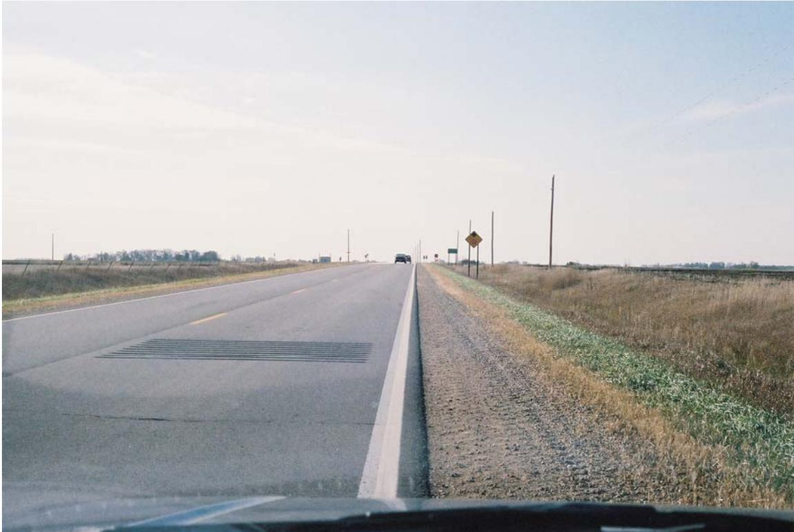
Photograph #155 (Reel #8, 2) (from East, looking West): first rumble strip and warning sign in view.
