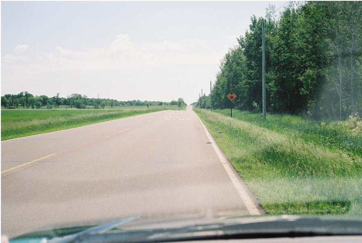
Photograph #226 (Reel #11, 12A) (from North, looking South): first rumble strip *missing*; warning sign in view; STOP AHEAD on road.
