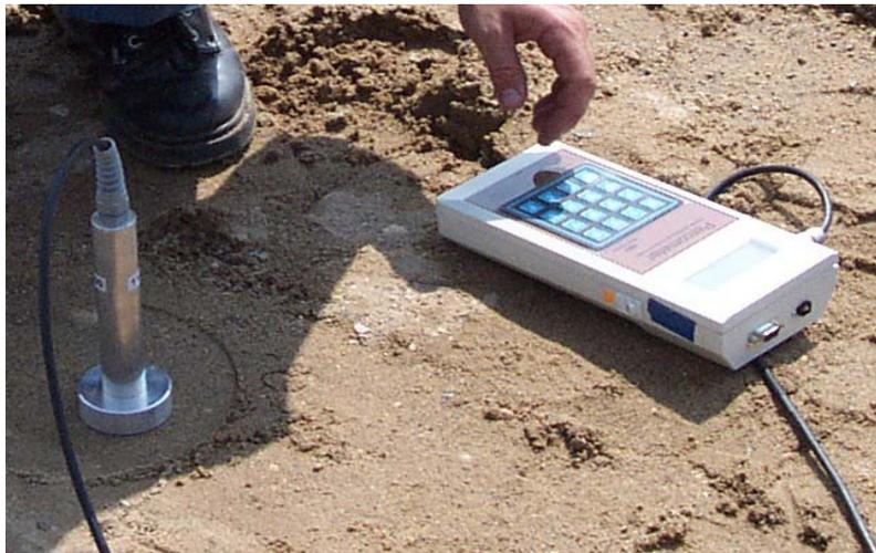
Fig. 3.6 Percometer
