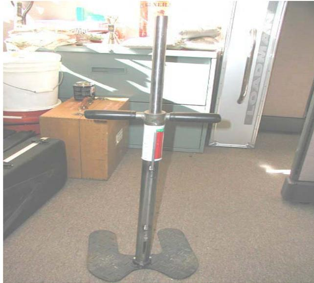
Figure 3.9 Rapid Compaction Control Device
