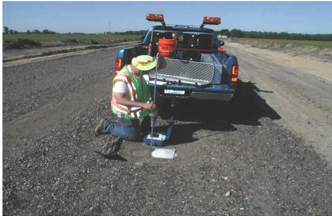
Figure 3.3b An example of DCP testing
