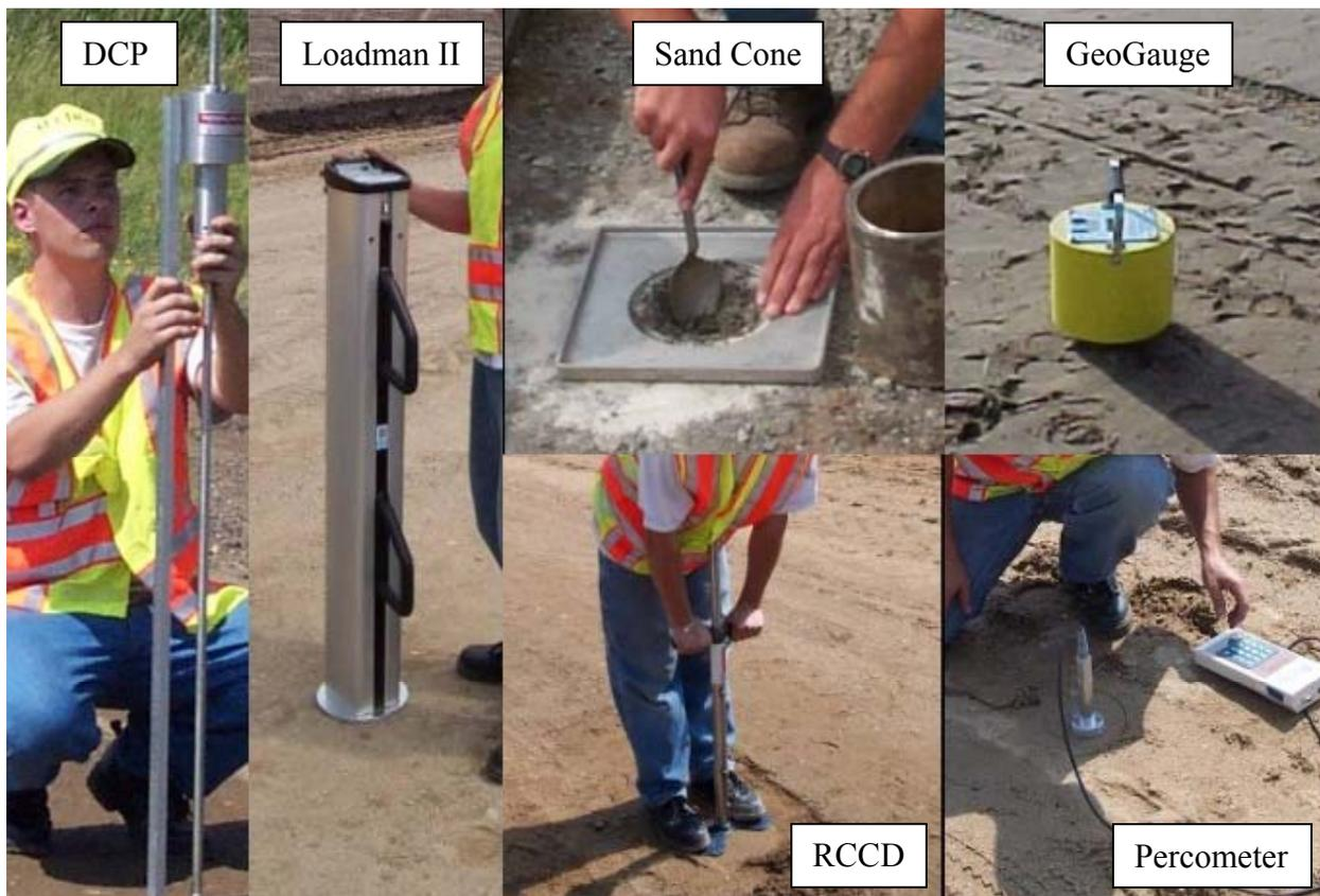
Figure 1. Test equipment used during the 2002 construction season.
