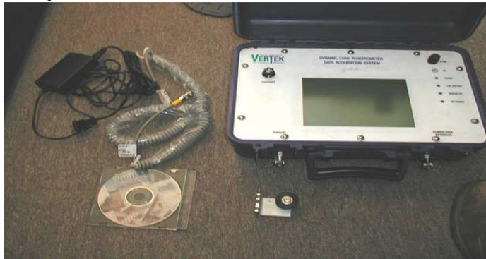
Fig.3.4 Automatic DCP data acquisition system
