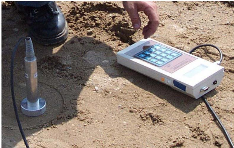
Fig. 3.6 Percometer
