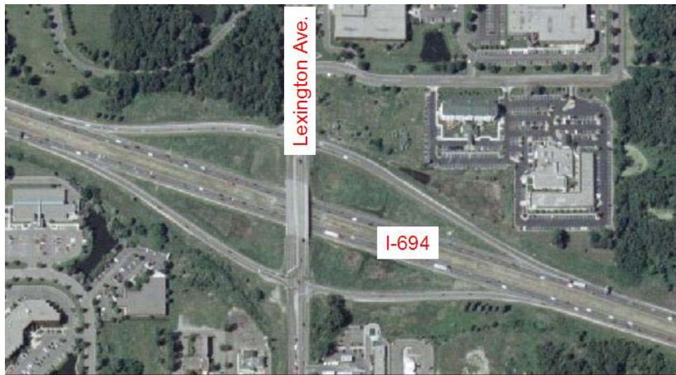
Figure 5-1. Diamond interchange at Lexington Avenue and I-494
