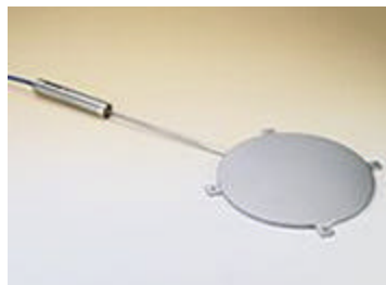
Figure 3.3. Geokon model 4800 earth pressure cell ( www.geokon.com ).
