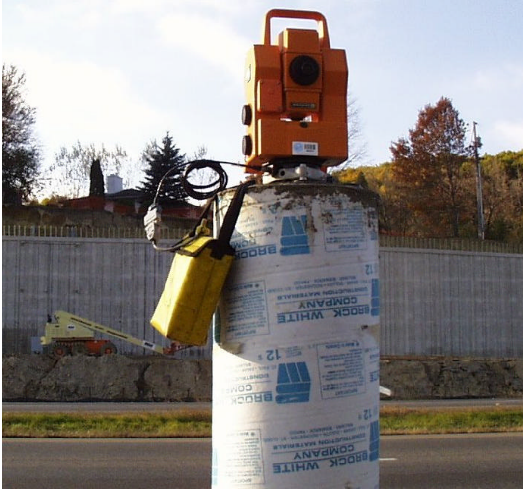
Figure 3.10. Total station mounted on concrete monument.
