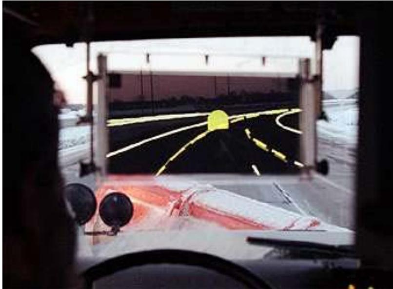
**Figure 2-2: HUD display under bright conditions. Note the lack of glare through the combiner.**
