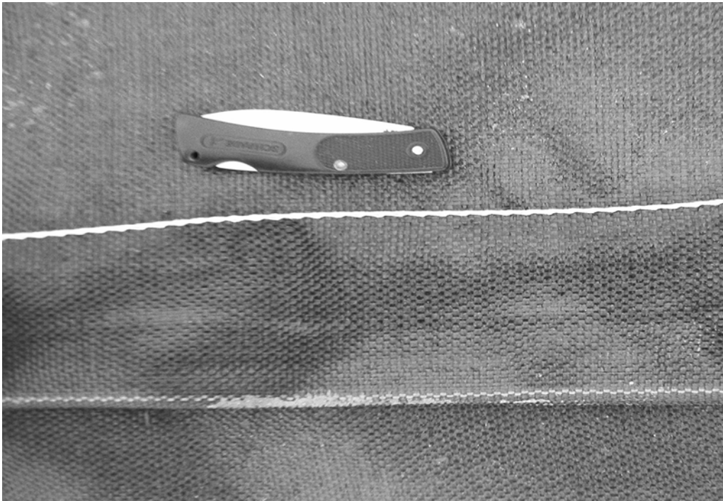
Figure 4.6 Type V Woven Geofabric Connected Using a “Prayer seam” with 75-mm (3-in.) Overlap and 401 Stitch.
