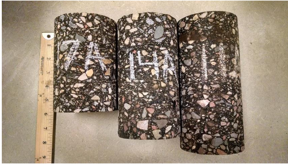
Figure 4-16 TH 47 (2014) cores used for RM (Cores 11, 14, and 17)
