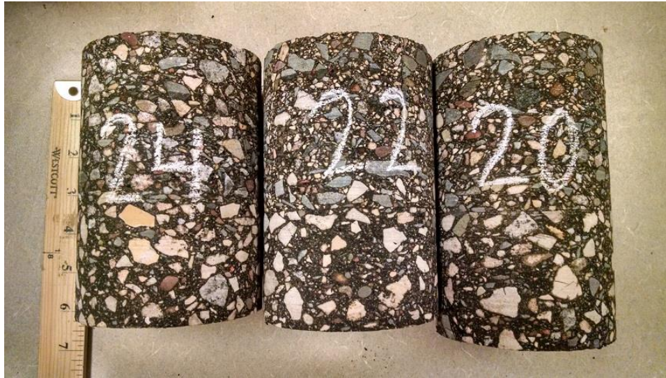
Figure 4-14 TH 36 (2008) cores used for RM (Cores 20, 22, and 24)
