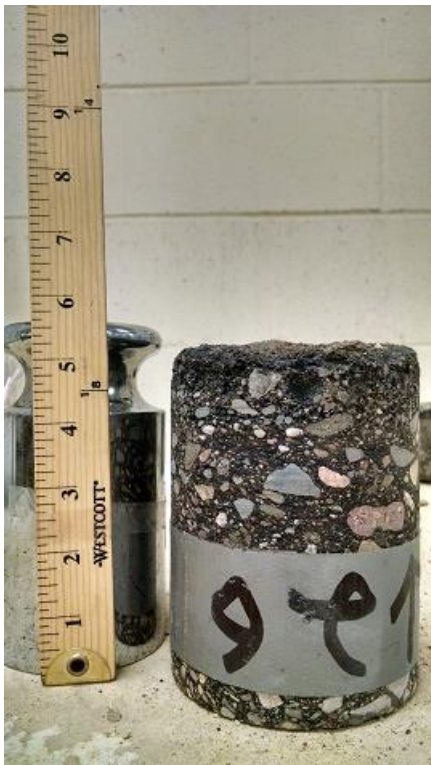
Figure A-17 Core 26, TH 95 (2013), un-cracked, non-wheelpath
