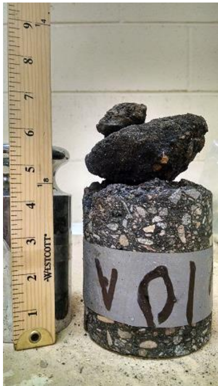
Figure A-25 Core 10; TH 47 (2014), cracked, wheelpath
