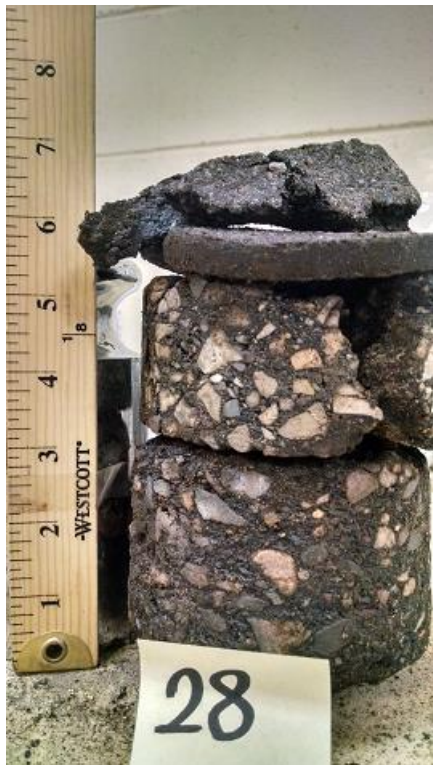
Figure A-19 Core 28, TH 95 (2013), cracked, wheelpath
