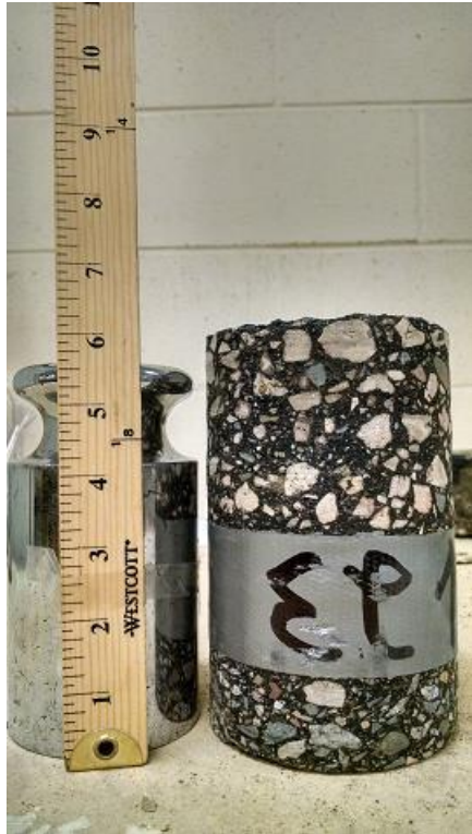
Figure A-14 Core 23, TH 36 (2008), un-cracked, non-wheelpath
