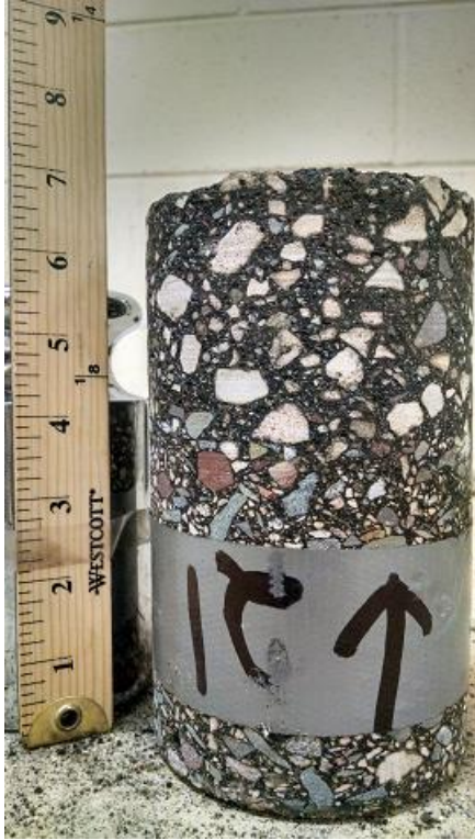
Figure A-12 Core 21, TH 36 (2008), un-cracked, non-wheelpath
