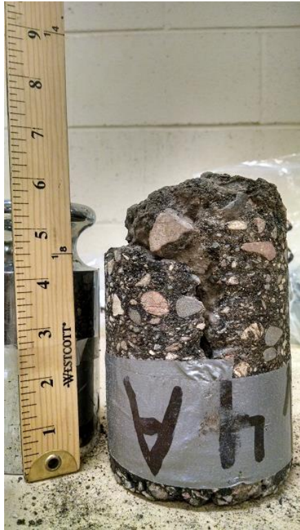
Figure A-4 Core 4, TH 10 (2004), cracked, wheelpath
