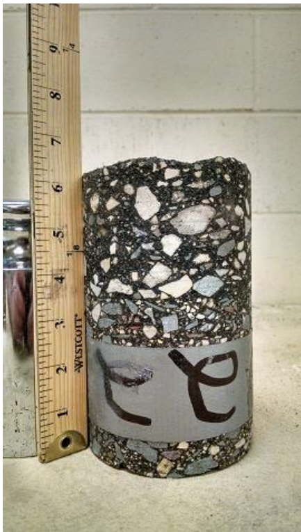
Figure A-13 Core 22, TH 36 (2008), un-cracked, wheelpath
