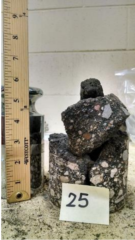
Figure A-16 Core 25; TH 95 (2013), cracked, wheelpath
