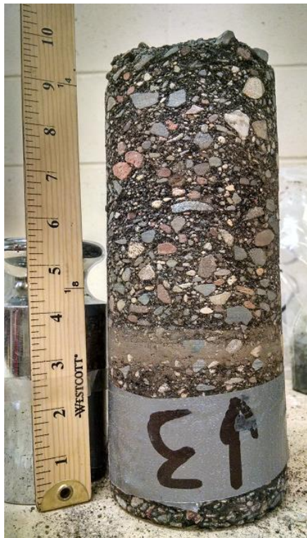
Figure A-3 Core 3, TH 10 (2004), un-cracked, wheelpath
