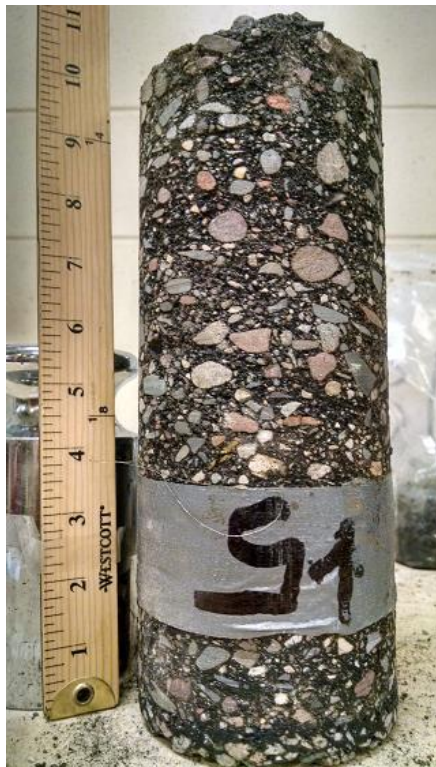
Figure A-5 Core 5, TH 10 (2004), un-cracked, non-wheelpath
