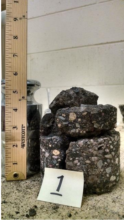
Figure A-1 Core 1; TH 10 (2004), cracked, wheelpath
