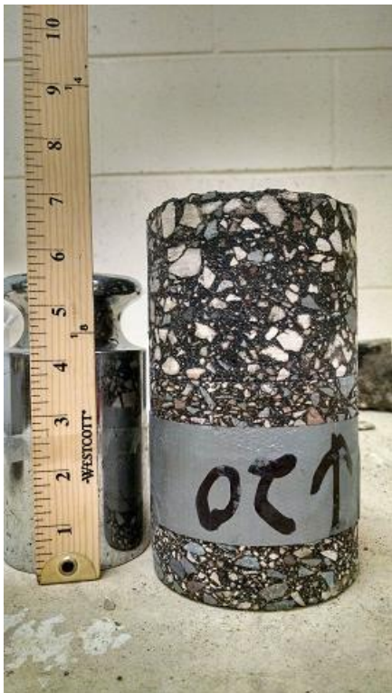
Figure A-11 Core 20, TH 36 (2008), un-cracked, wheelpath
