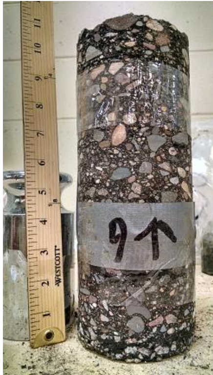
Figure A-6 Core 6, TH 10 (2004), un-cracked, wheelpath
