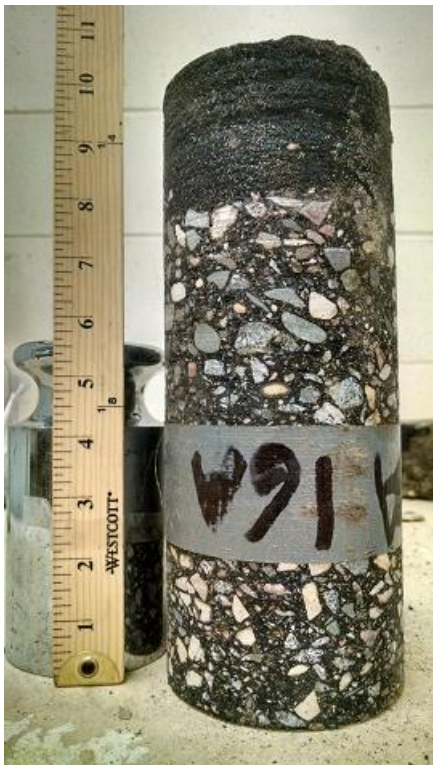
Figure A-31 Core 16, TH 47 (2014), cracked, wheelpath
