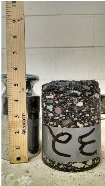
Figure A-23 Core 32, TH 95 (2013), un-cracked, non-wheelpath
