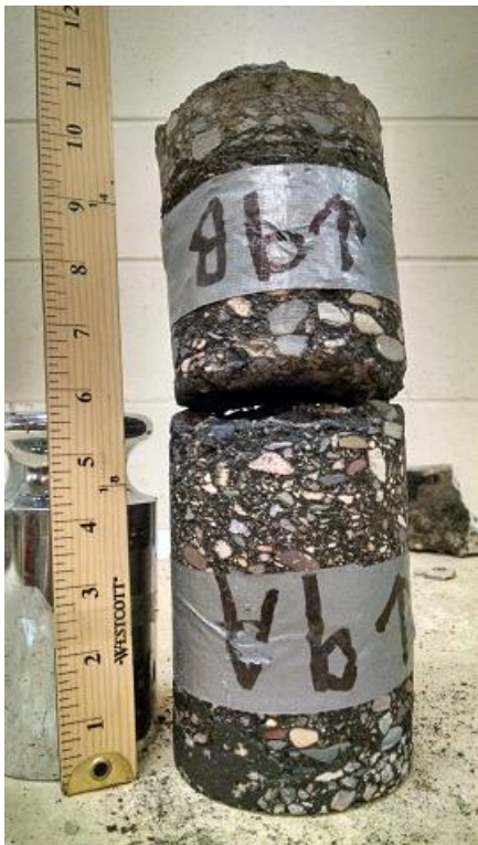
Figure A-9 Core 9, TH 10 (2004), un-cracked, wheelpath
