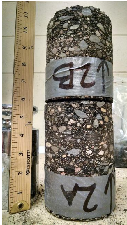
Figure A-2 Core 2, TH 10 (2004), un-cracked, non-wheelpath
