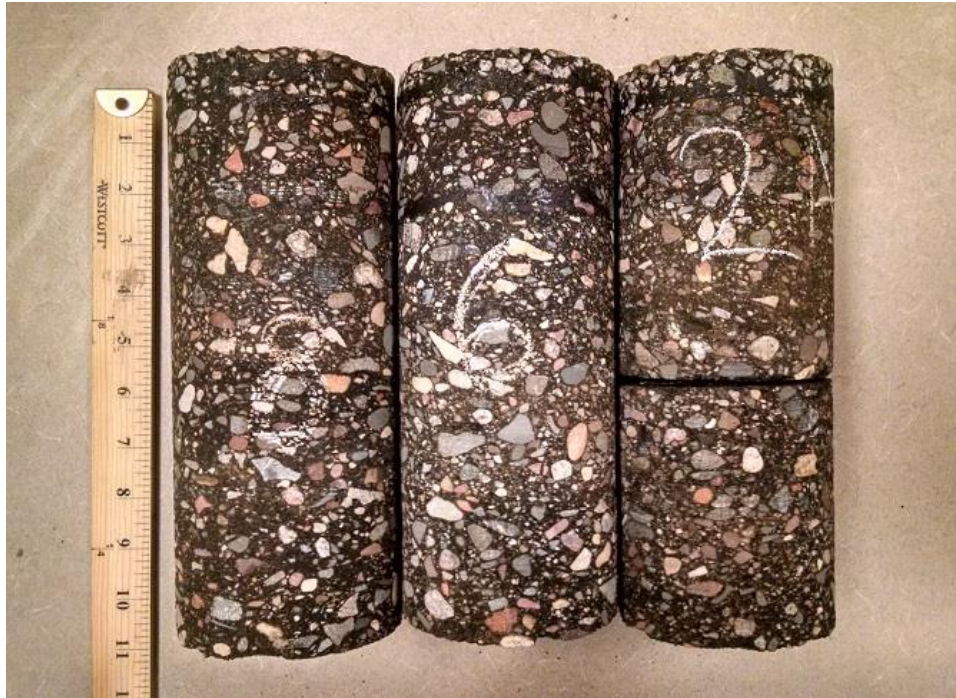
Figure 4-13 TH 10 (2004) cores used for RM (Cores 2, 6, and 8)
