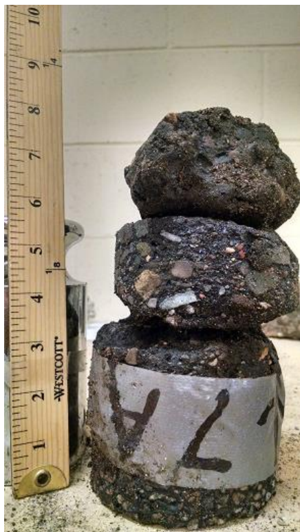
Figure A-7 Core 7, TH 10 (2004), cracked, wheelpath
