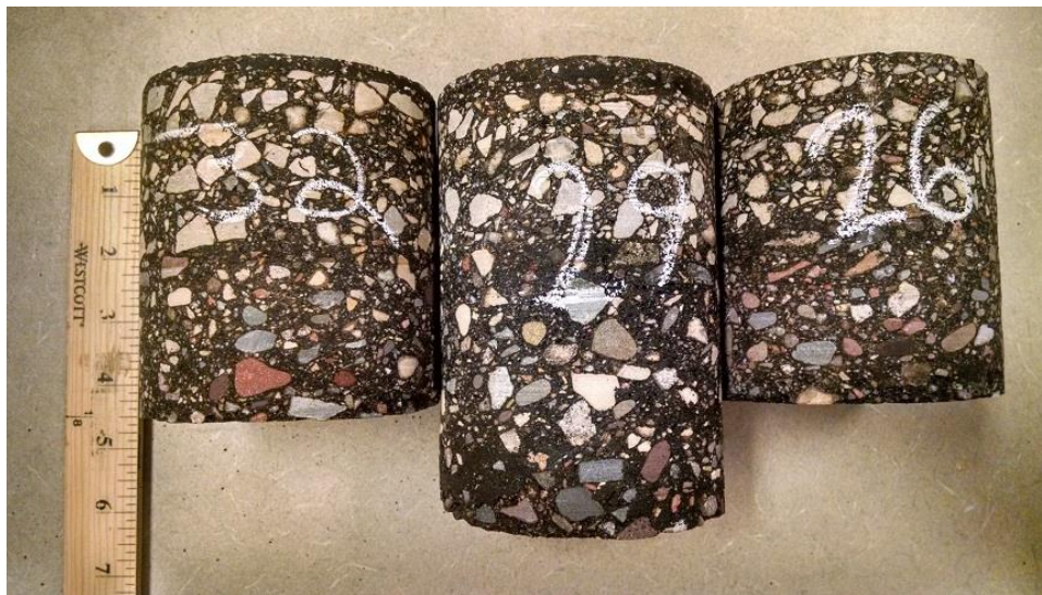
Figure 4-15 TH 95 (2013) cores used for RM (Cores 26, 29, and 32)
