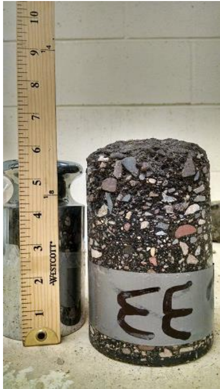
Figure A-24 Core 33, TH 95 (2013), un-cracked, wheelpath
