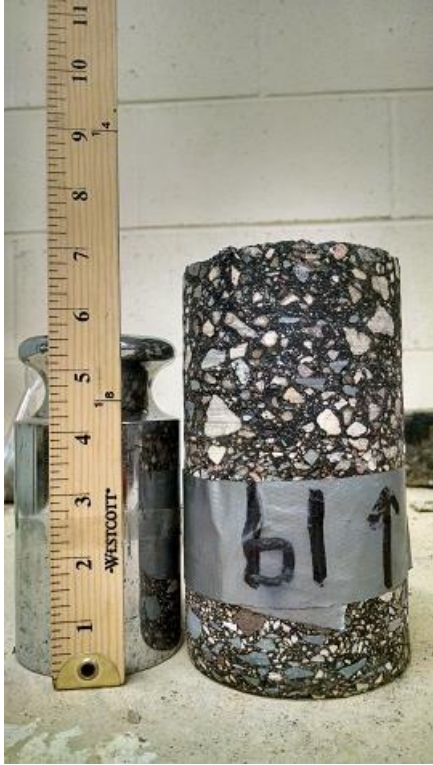
Figure A-10 Core 19, TH 36 (2008), un-cracked, non-wheelpath
