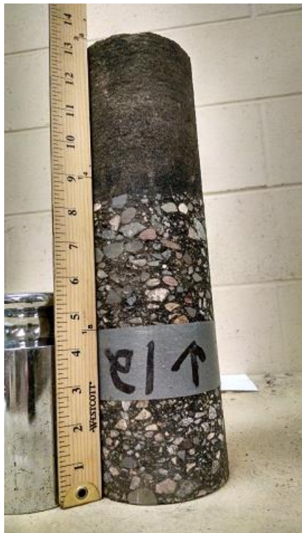
Figure A-27 Core 12, TH 47 (2014), un-cracked, wheelpath
