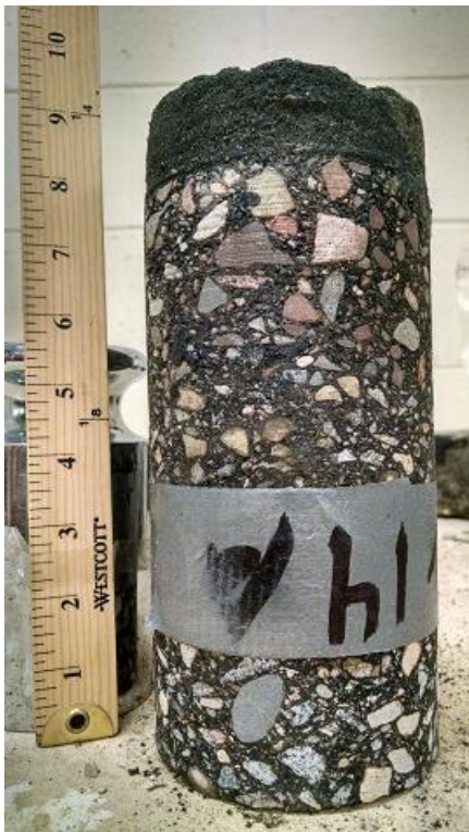
Figure A-29 Core 14, TH 47 (2014), un-cracked, non-wheelpath
