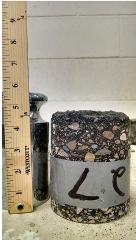
Figure A-18 Core 27, TH 95 (2013), un-cracked, wheelpath
