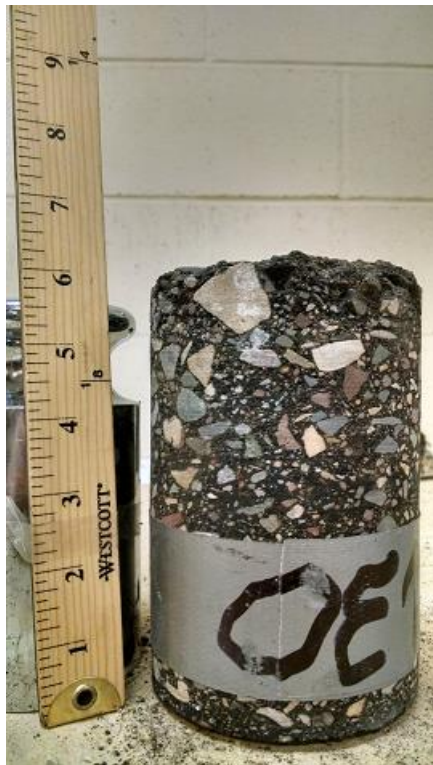
Figure A-21 Core 30, TH 95 (2013), un-cracked, wheelpath
