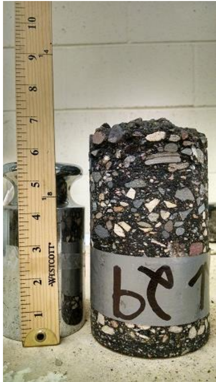
Figure A-20 Core 29, TH 95 (2013), un-cracked, non-wheelpath
