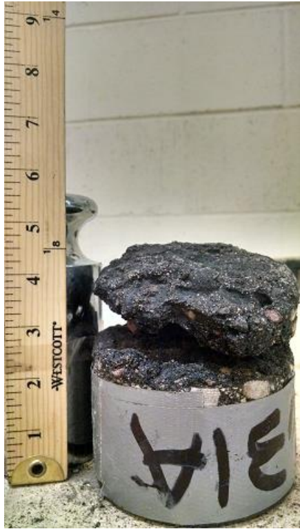
Figure A-22 Core 31, TH 95 (2013), cracked, wheelpath
