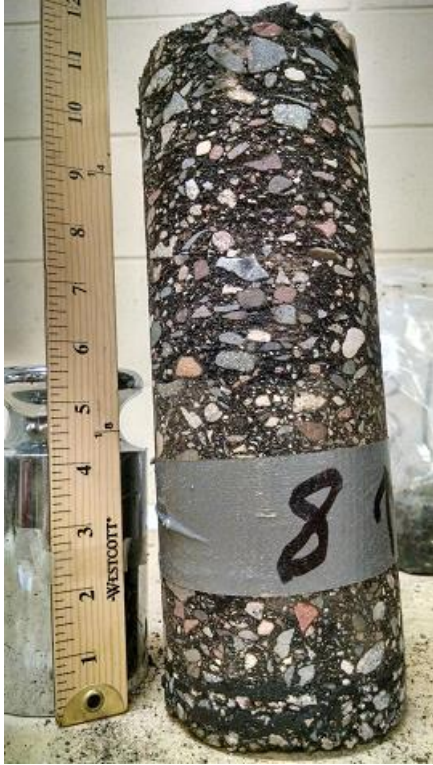
Figure A-8 Core 8, TH 10 (2004), un-cracked, non-wheelpath
