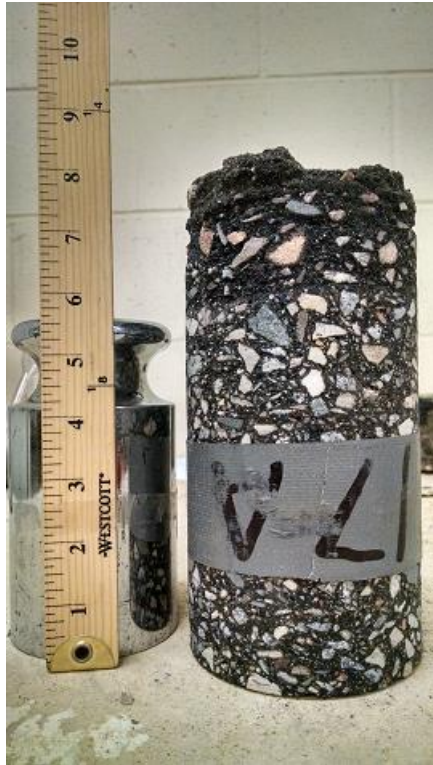
Figure A-32 Core 17, TH 47 (2014), un-cracked, non-wheelpath
