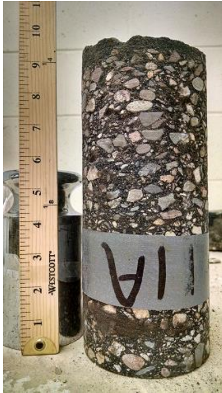
Figure A-26 Core 11, TH 47 (2014), un-cracked, non-wheelpath
