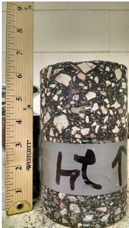
Figure A-15 Core 24, TH 36 (2008), un-cracked, wheelpath
