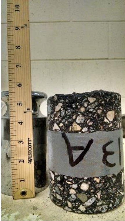
Figure A-28 Core 13, TH 47 (2014), cracked, wheelpath
