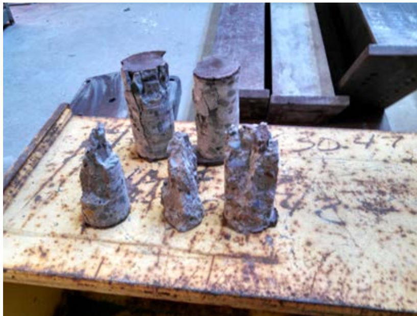
Figure F.4: Failed core samples from Bridges 27799L and 62834
