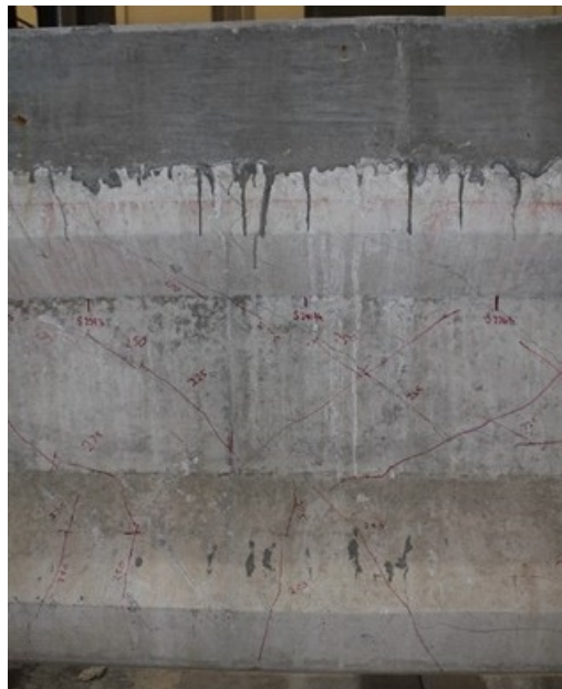
Figure F.18: Photograph of Bridge 62384 girder (End B) at end of test showing first observed shear cracks, which occurred near applied load in long shear span
