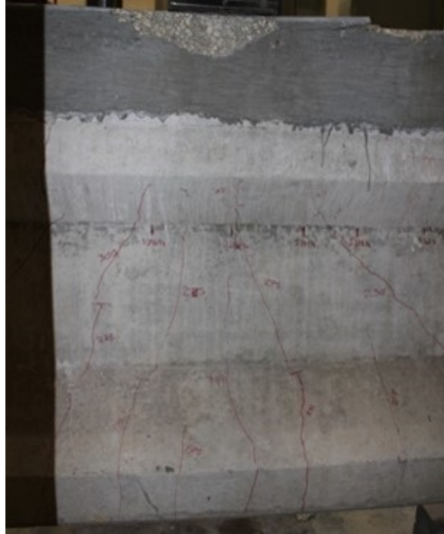
Figure F.19: Photograph of Bridge 62384 girder (End B) at end of test showing flexural cracks observed below applied load
