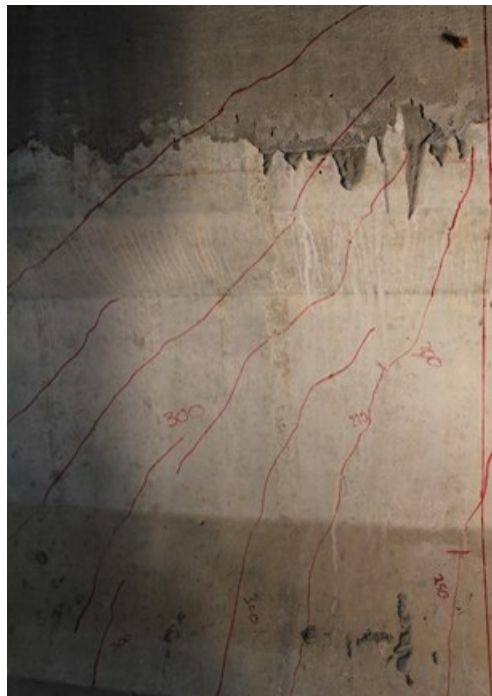
Figure F.14: Photograph of Bridge 62834 girder (End A) at end of test showing flexural cracks observed below applied load
