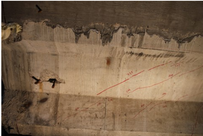
Figure F.10: Photograph of Bridge 27799L girder at end of test showing first shear cracks observed near support in short shear span
