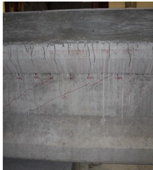
Figure F.20: Photograph of Bridge 62384 girder (End B) at end of test showing first shear cracks observed near support in short shear span
