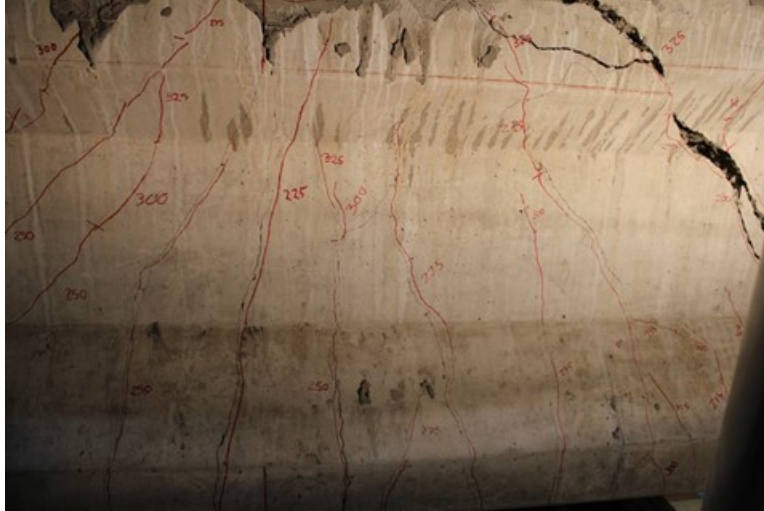
Figure F.9: Photograph of Bridge 27799L girder at end of test showing flexural cracks observed below the applied load
