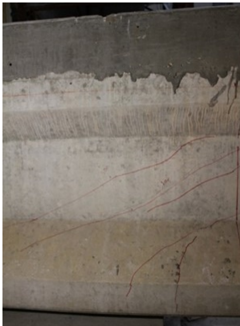
Figure F.16: Photograph of Bridge 62384 girder (End A) at end of test showing first shear cracks observed near support in short shear span
