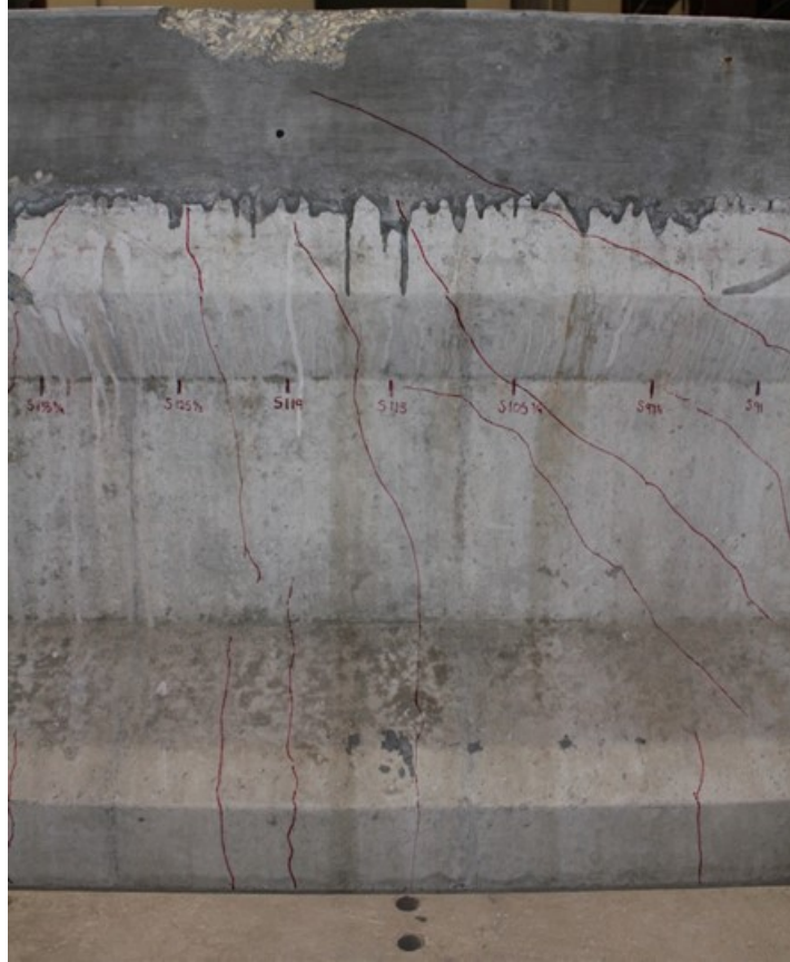
Figure F.21: Photograph of Bridge 62384 girder (End B) at onset of deck concrete crushing
