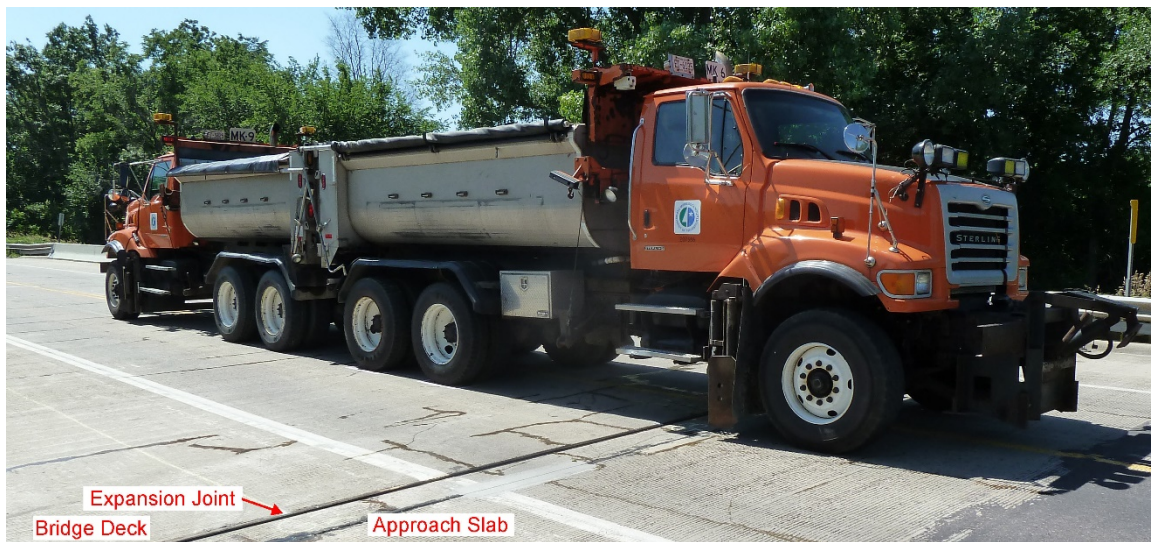
Figure 6.3: Back-to-back truck position
