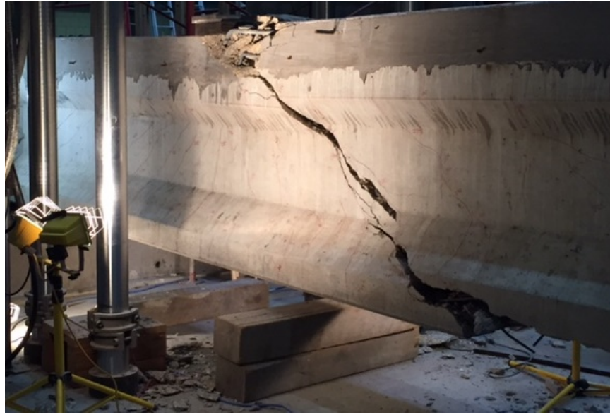
Figure F.11: Failure of Bridge 27799L girder in flexure-shear
