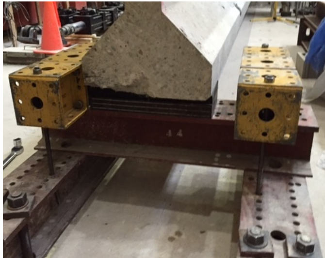
Figure F.6: Typical girder support boundary conditions
