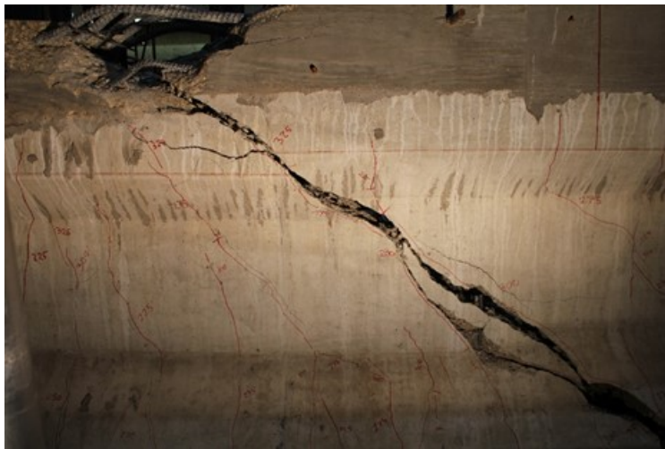
Figure F.8: Photograph of Bridge 27799L girder at end of test showing first observed shear crack, which occurred near applied load in long shear span (labeled “200” kips)
