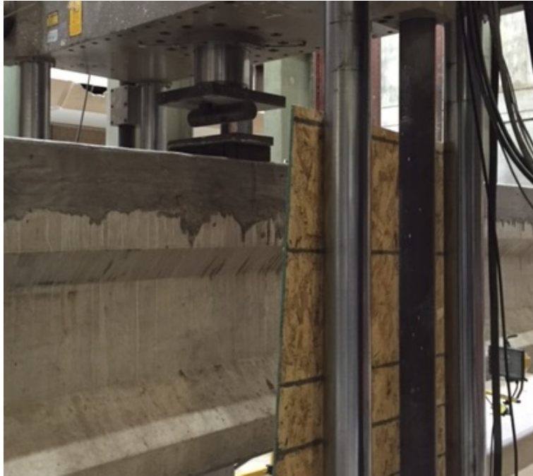
Figure F.5: Typical point load boundary conditions
