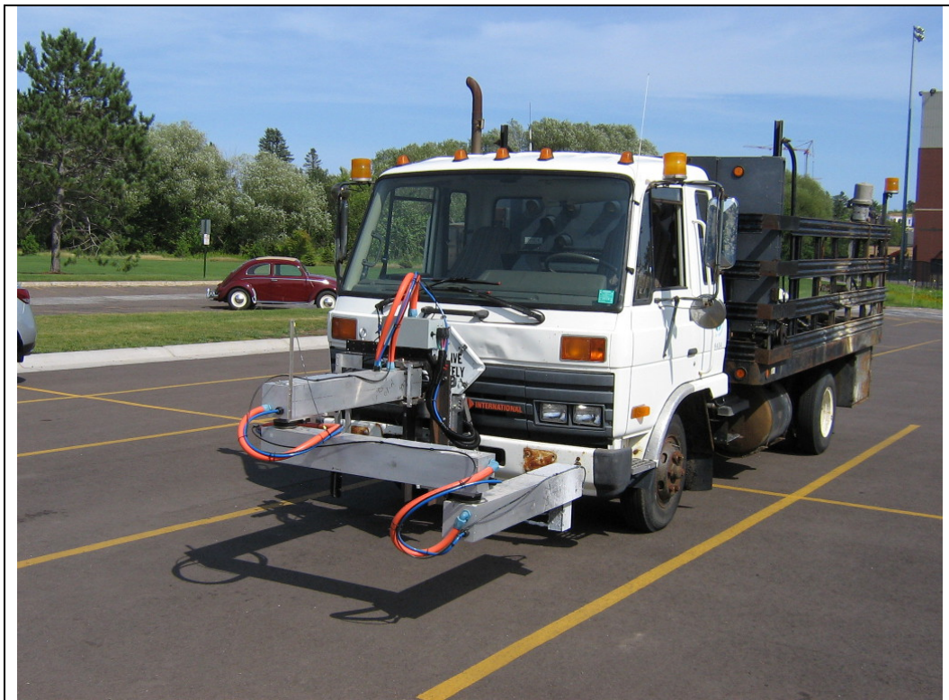
Figure 2.21. Truck-mounted robot arm deployed for testing.
