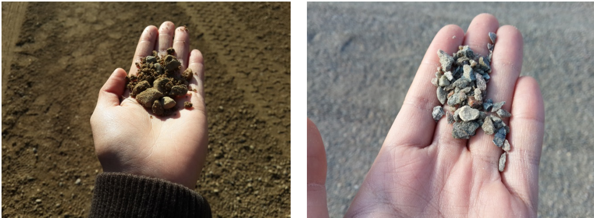
Figure 29. Beltrami County Angularity Comparison between Standard Class 1 (left) and Crusher Dust (right)
