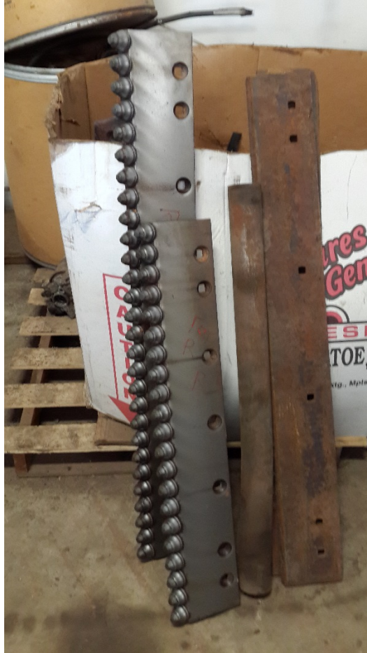
Figure 3. Carbide-Tipped Blades on the Left
