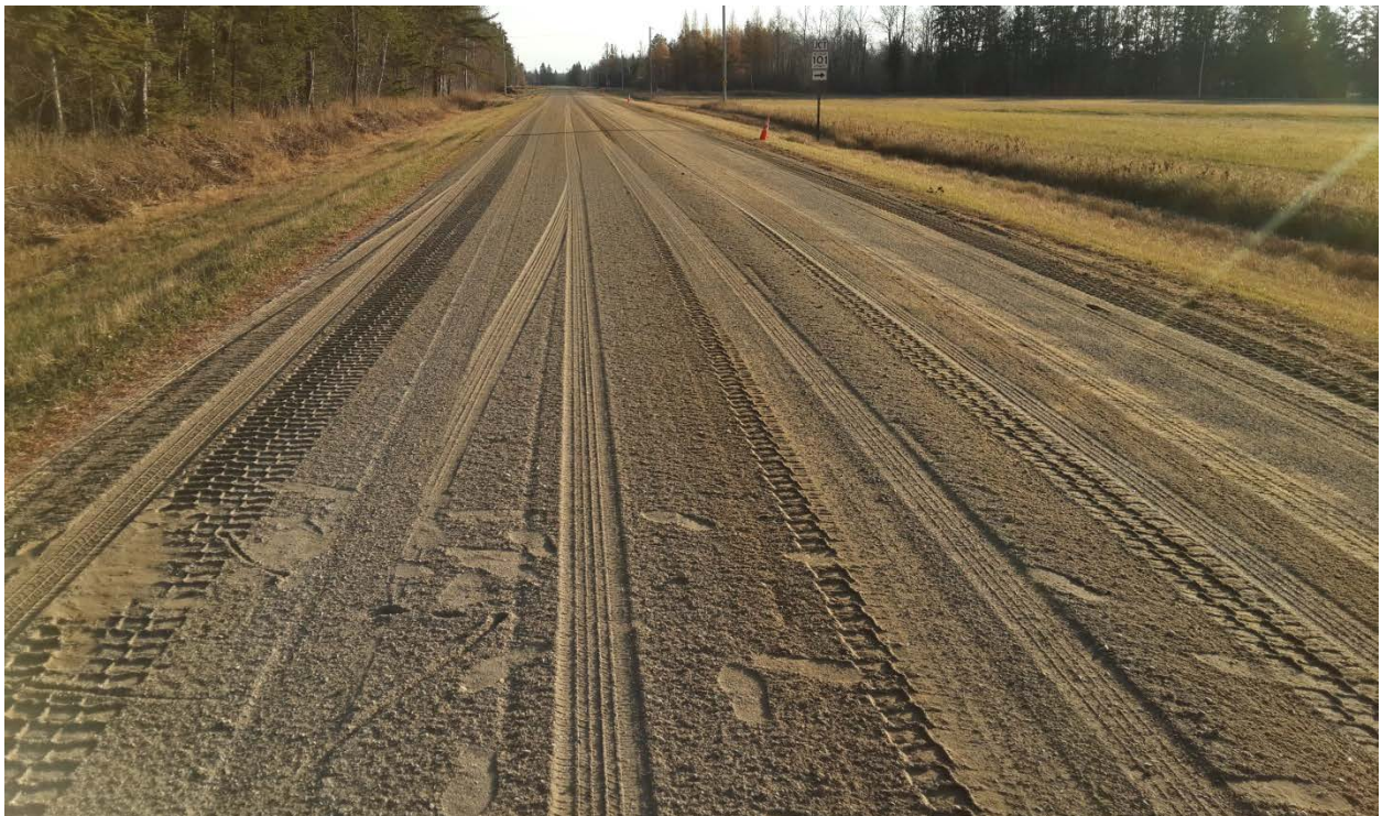
Figure 27. Beltrami County CR 23 Middle Test Section (83 Tons of Crusher Dust)
