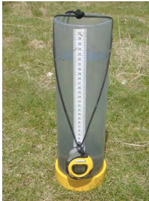
Figure 3. Picture of a Modified Philip Dunne (MPD) infiltrometer.
