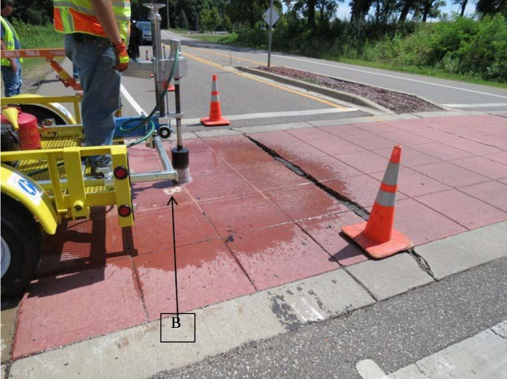
Figure 4.55 Crosswalk on westbound lane of Lake Johanna Blvd. in Arden Hills. Due to access limitations, core samples were taken from a neighboring joint line.
