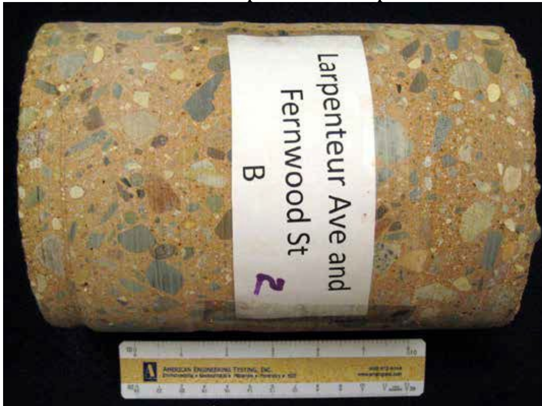
L&F B DESCRIPTION: Traffic-worn top surface of the core sample as received.
