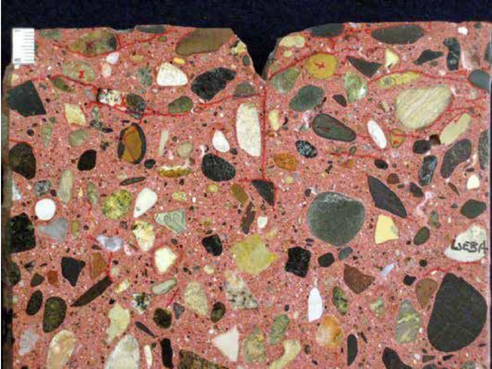
Figure 4.60 Arden Hills - Core sample LJEB-A showing clear ASR gel product within microcracks traversing both the paste and a greywacke coarse aggregate particle
