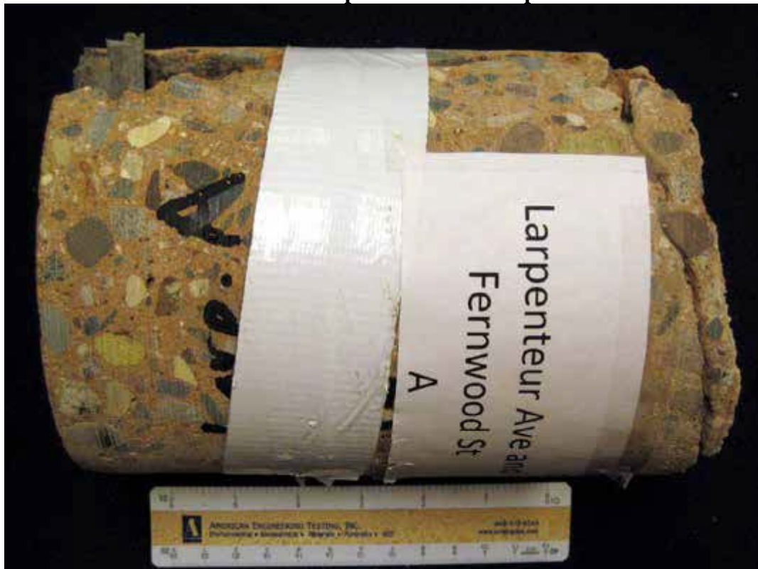
L&F A DESCRIPTION: Core sample as received. Top surface is left.
