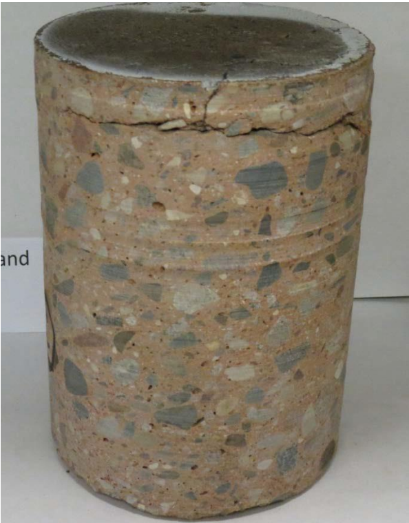
Figure 4.80 Roseville - Core sample L&F- C showing vertical crack up from horizontal delamination crack
