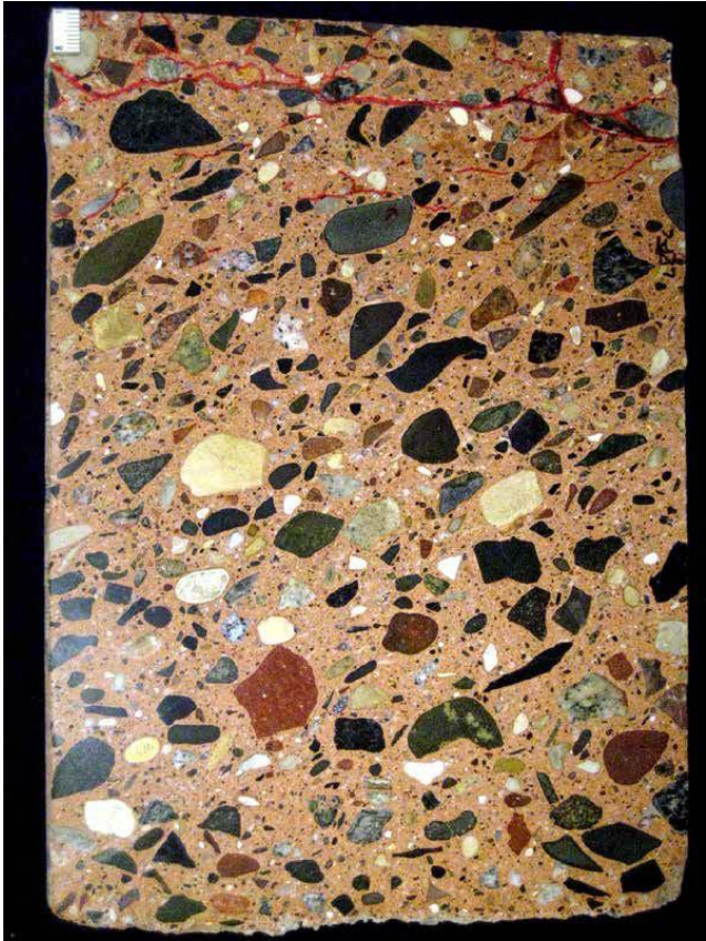
Figure 4.82 Roseville - Core sample L&F-C showing ASR gel product (highlighted in red ink) within microcracks traversing the paste, fine and coarse aggregate particles
