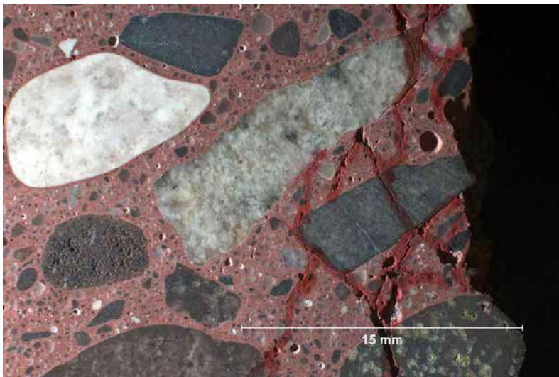
Figure 4.50 Vadnais Heights - Core sample 96D. Note microcracking near joint face (highlighted in red ink)
