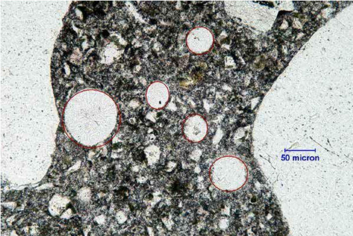
Figure 4.52 Vadnais Heights - Core sample 96D showing darker, low w/cm paste, indicating multiple additions of water during batching
