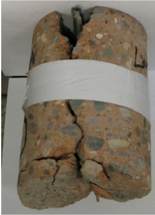
Figure 4.73 Roseville - Core sample L&F-A showing carbonation (unstained paste) proceeding up to 10mm depth from the joint crack plane (on right)
