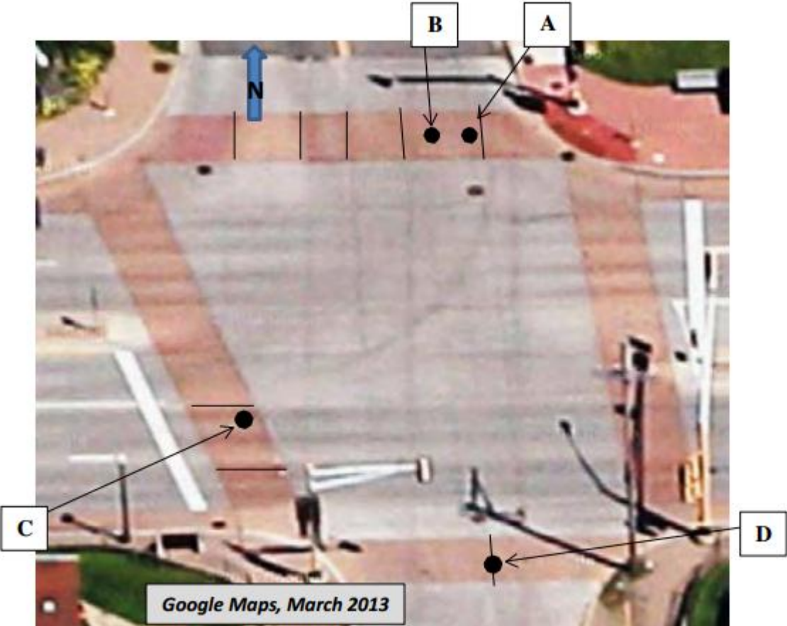
Figure 4.68 Overhead view of Larpenteur Avenue and N Fernwood Street intersection indicating locations where core samples were extracted
