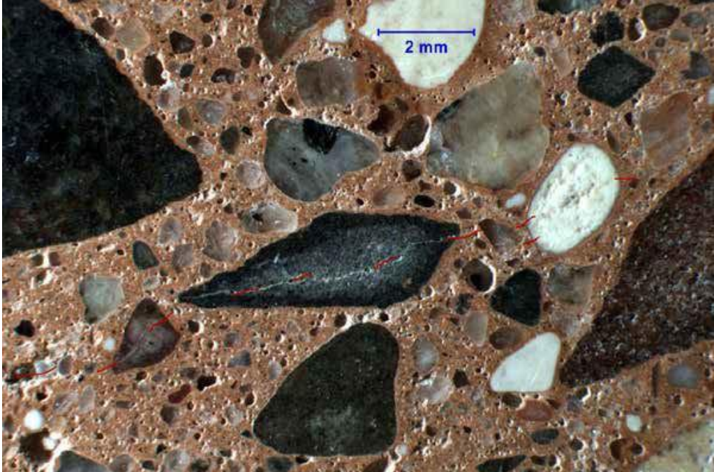
Figure 4.82 Roseville - Core sample L&F-C showing ASR gel product (highlighted in red ink) within microcracks traversing the paste, fine and coarse aggregate particles
