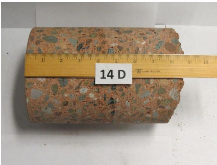
Figure 4.19 Centerville - Core 14D showing good condition throughout depth
