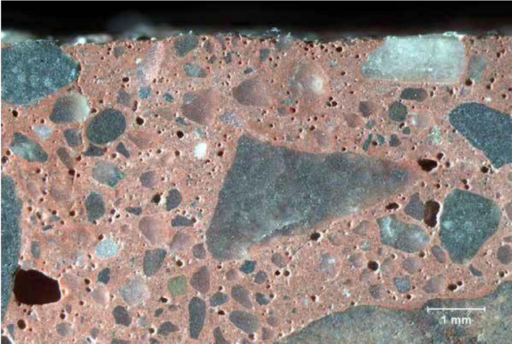
Figure 4.35 Vadnais Heights - Core sample 96A showing unfilled air voids near top of pavement
