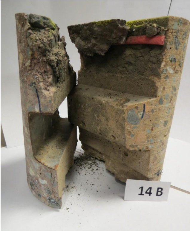
Figure 4.5 Keyed longitudinal joint between two different color sections
