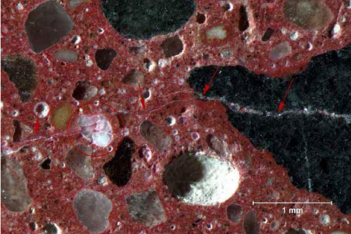
Figure 4.60 Arden Hills - Core sample LJEB-A showing clear ASR gel product within microcracks traversing both the paste and a greywacke coarse aggregate particle
