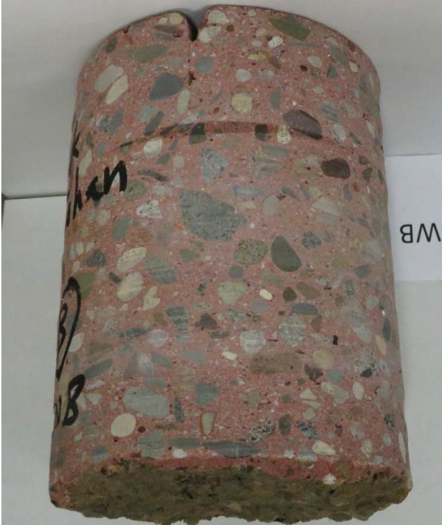
Figure 4.63 Arden Hills - Core sample LJWB-B showing vertical and horizontal ASR-induced cracks (highlighted in red ink)
