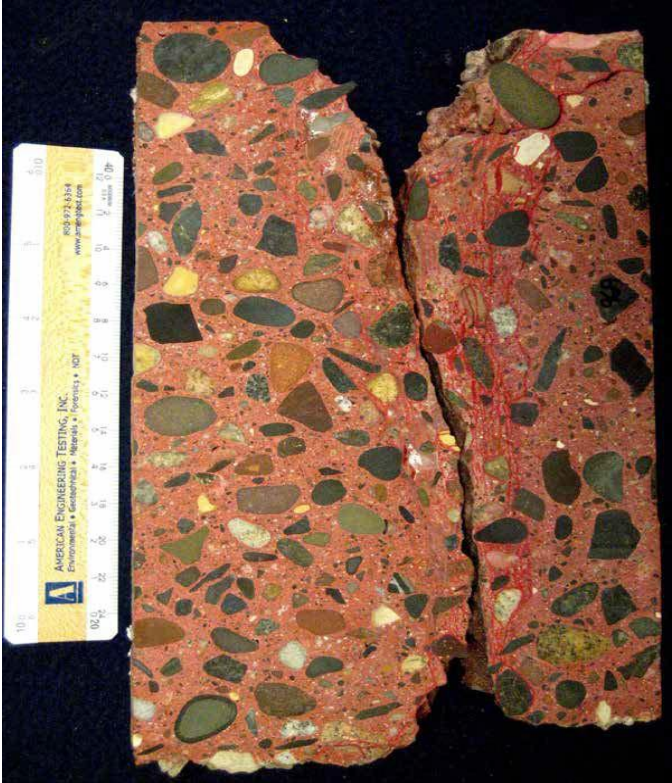
Figure 4.35 Vadnais Heights - Core sample 96A showing unfilled air voids near top of pavement
