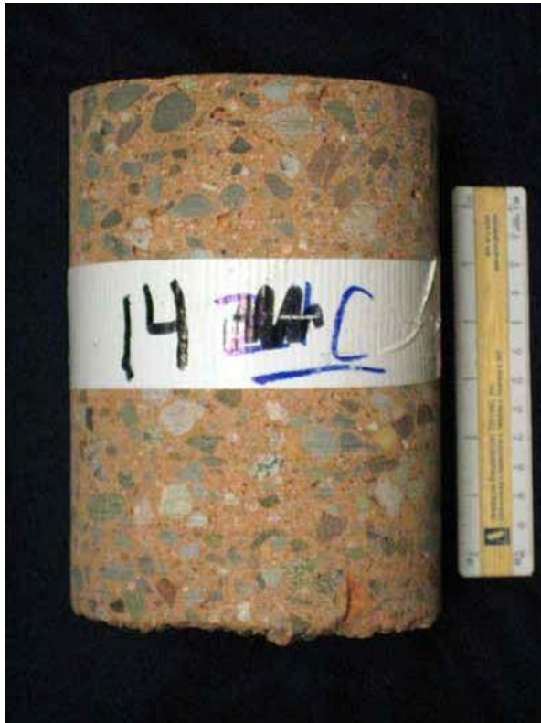
Figure 4.16 Centerville - Core 14C showing good condition throughout depth
