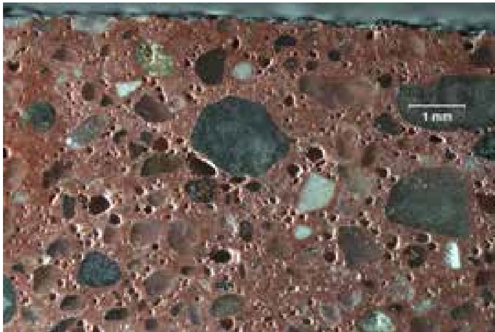
Magnification: 15x Description: Unfilled hardened air-void system at the top surface.
