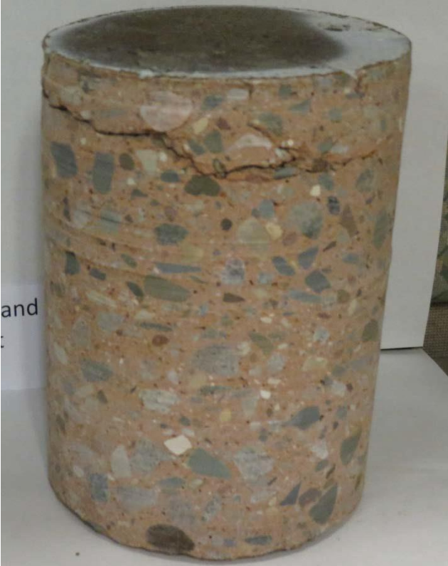
Figure 4.80 Roseville - Core sample L&F- C showing vertical crack up from horizontal delamination crack
