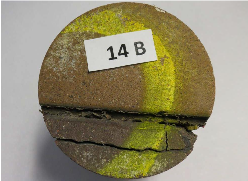
Figure 4.14 Centerville - Core 14B showing vertical cracks in darker colored side of joint near bottom of pavement
