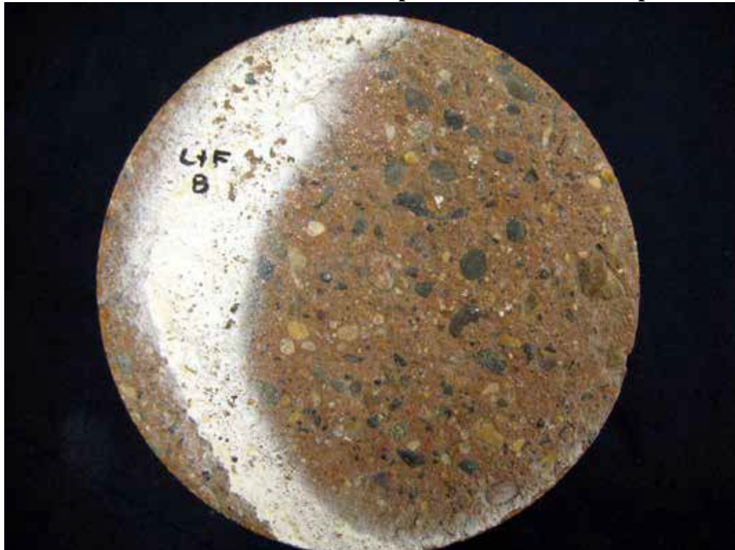
L&F B DESCRIPTION: Traffic-worn top surface of the core sample as received.
