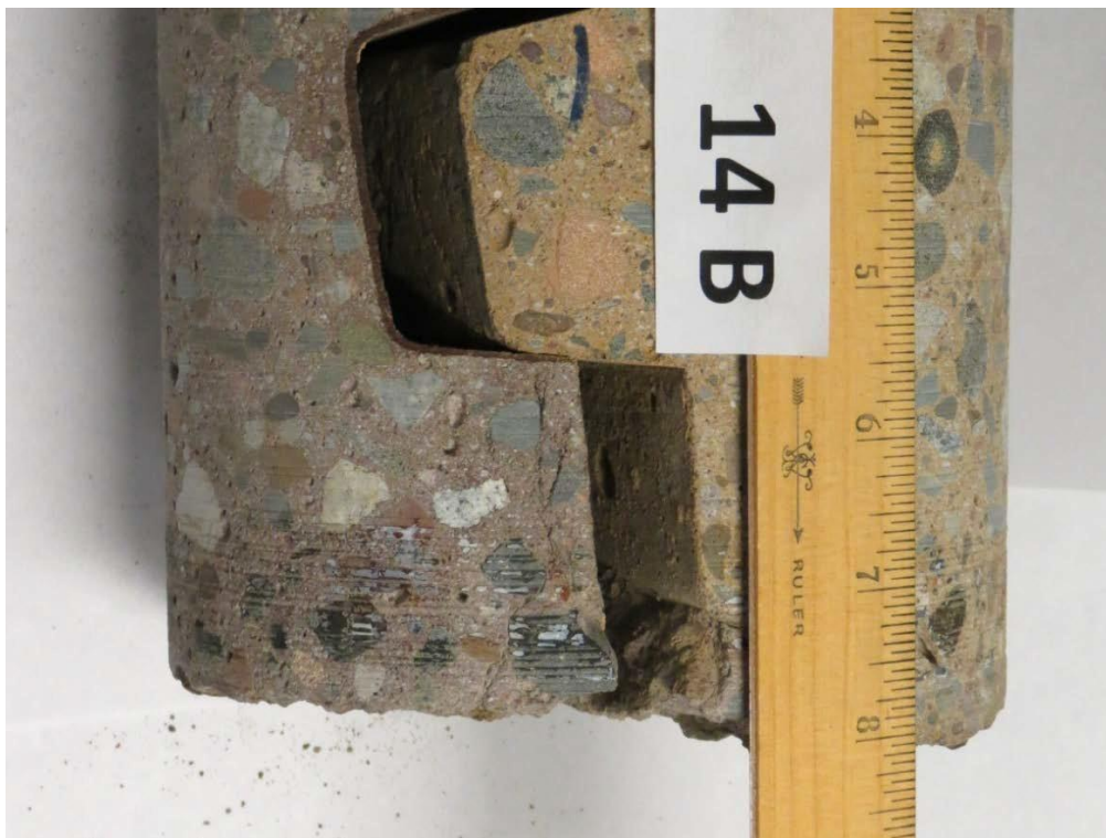
Figure 4.14 Centerville - Core 14B showing vertical cracks in darker colored side of joint near bottom of pavement
