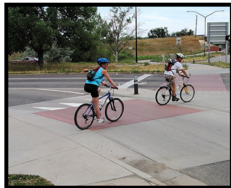
Figure 7.17 Channelized Turn Lane with Raised Crossing
