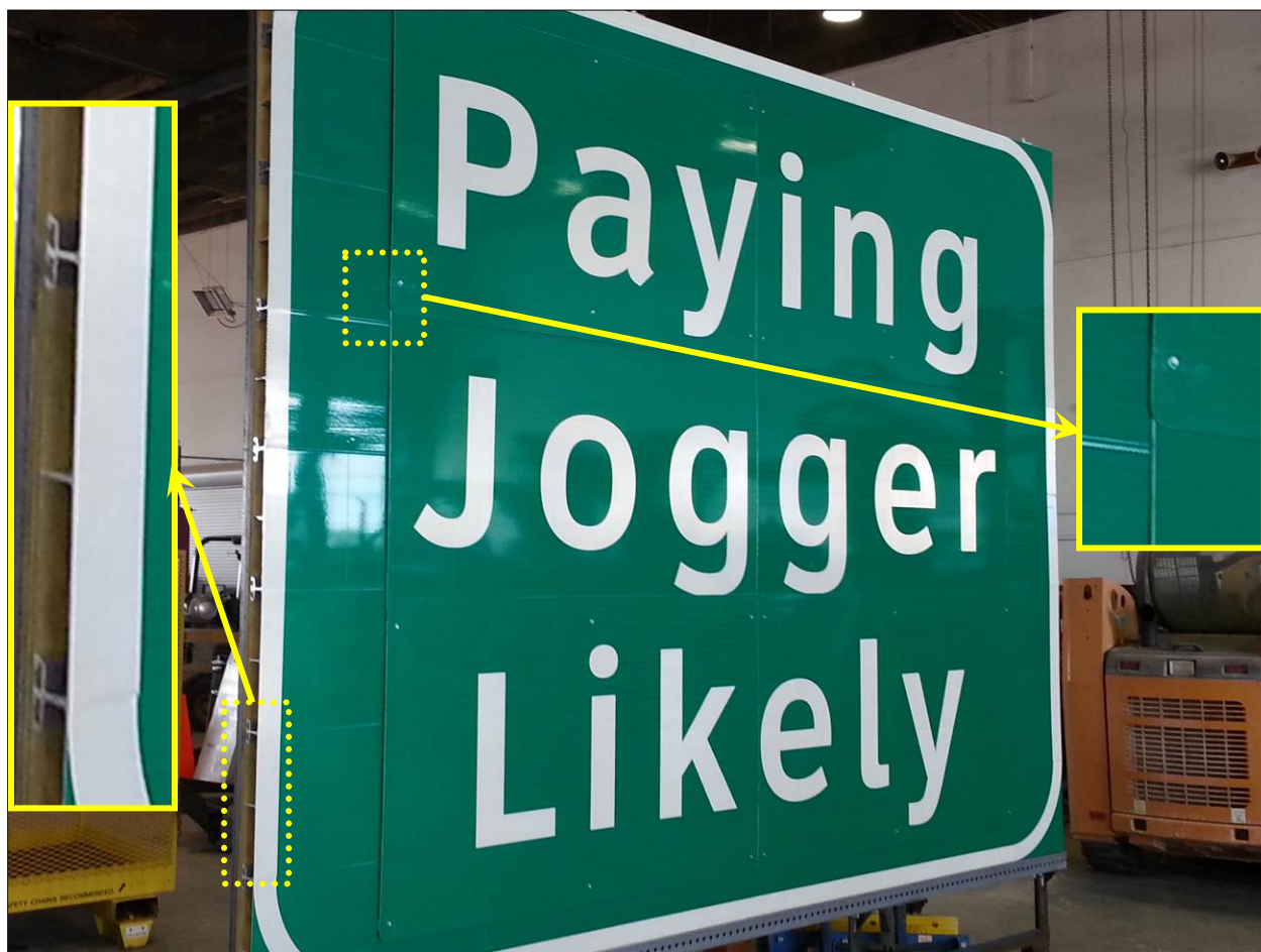
Figure 3.3. Overhead Guide Sign Construction.
