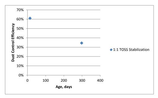
Figure 5 Dust control efficiency on Goodhue CR 52 Shingle Stabilization – 2013.
