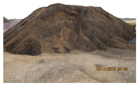
Figure 1 Jackson Co. 4 part shingles to 10 parts gravel blend, by volume
