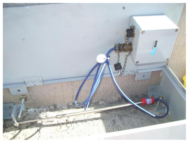
Figure 15: Sensors measuring relative displacements between barrier and wingwall.
