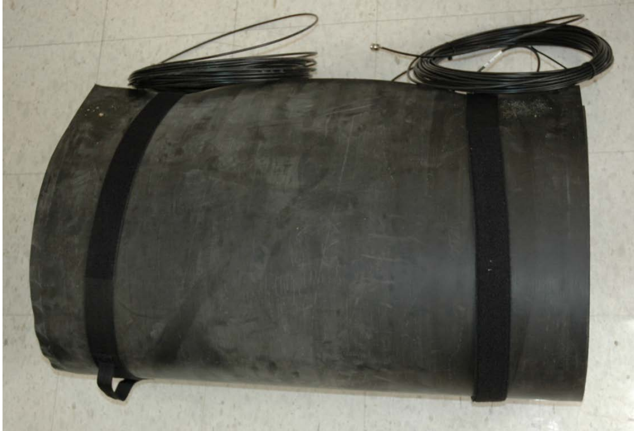
Figure 5: A single-lane, dual-strip weigh-pad prototype
