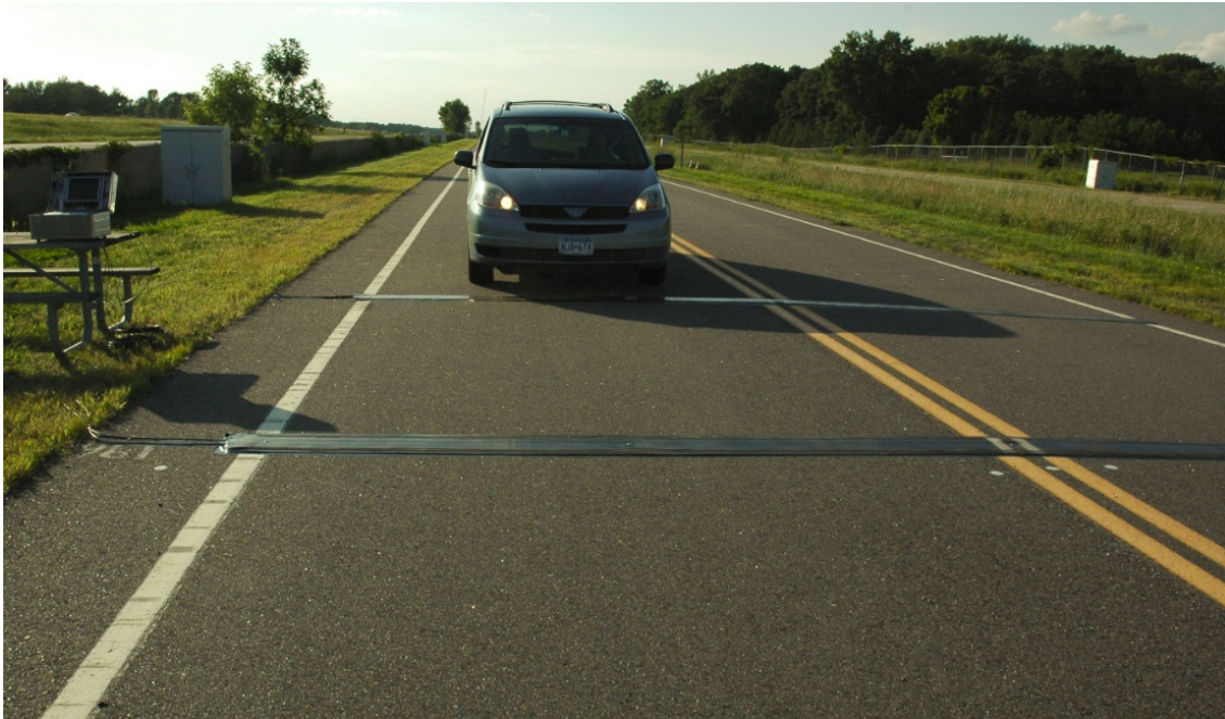
Figure 38: Installed weigh-pads with air cavity and the test vehicle
