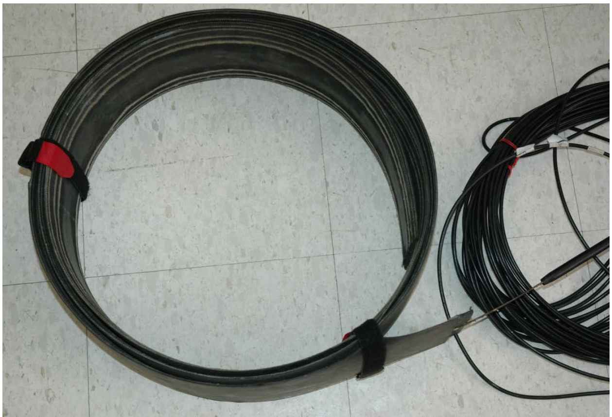
Figure 3: A single-lane, single-strip weigh-pad prototype
