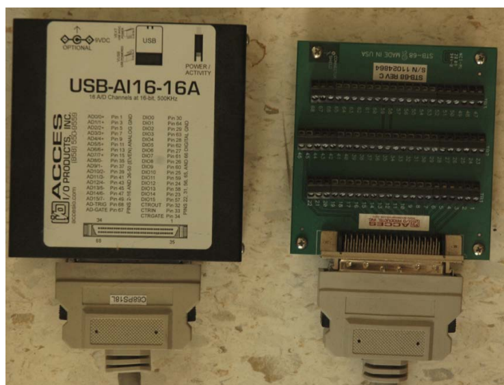
Figure 16: Access I/O Products Inc. USB-AI16-16A: 500K S/s, 16-bit ADC
