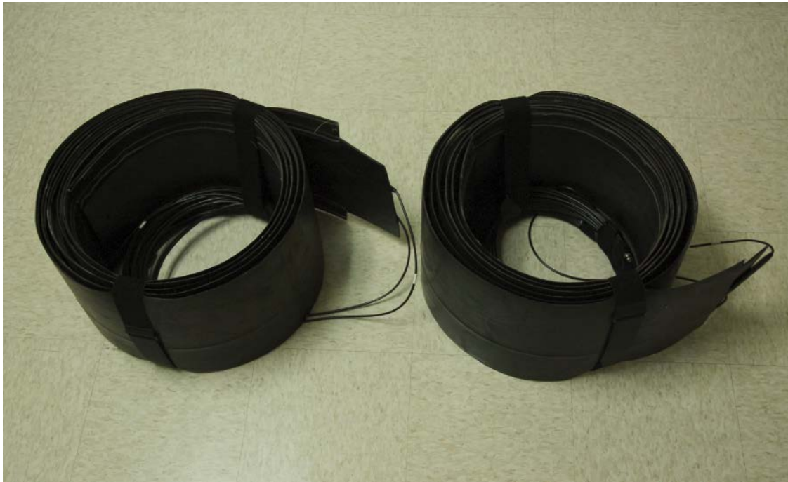
Figure 9: Prototypes of a pair of two-lane, single-strip weigh-pads
