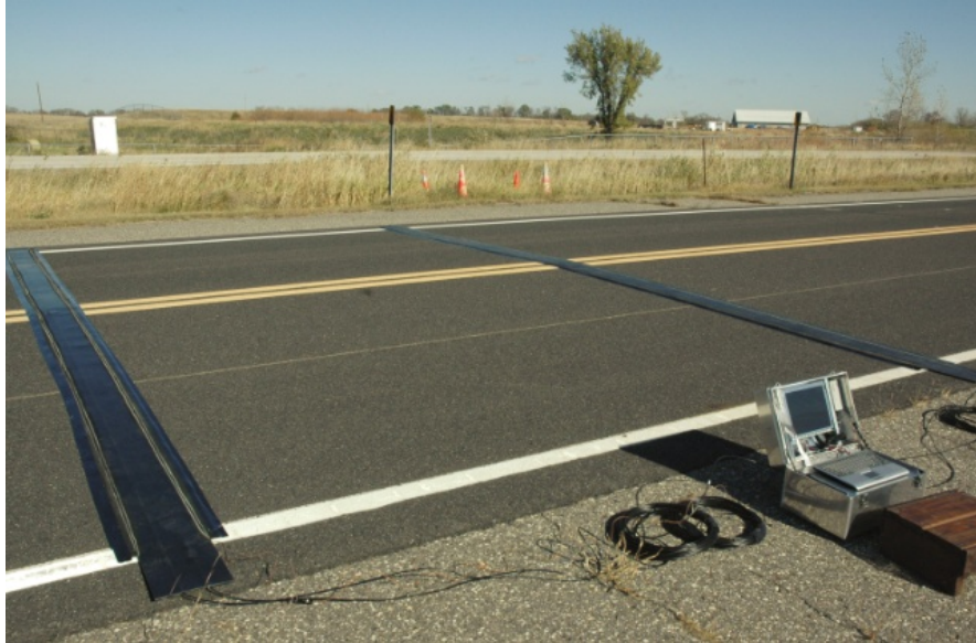
Figure 44: Speed effect test setup at MnRoad: the weigh-pads were fastened by high-strength tapes on leading and trailing edges and carpet tapes at the bottom
