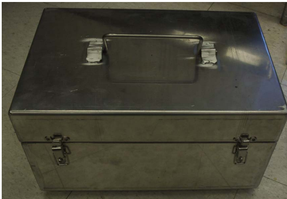
Figure 21: Custom enclosure built using aluminum sheets
