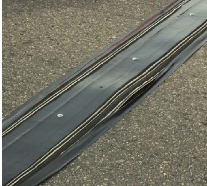
Figure 36: Some portions had wrinkles that caused vibration and error on the axle signal
