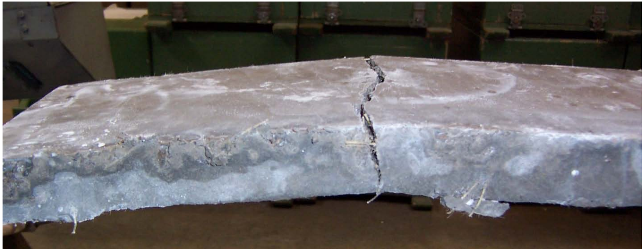
Figure 21: Thin Beam Failure 1
