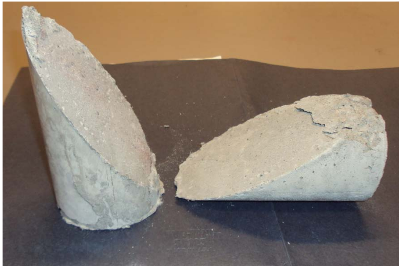
Figure 23: Failed Slant Shear Specimen
