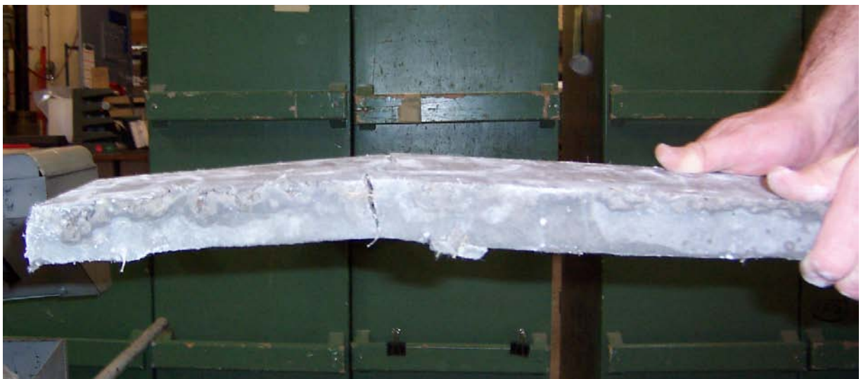
Figure 22: Thin Beam Failure 2
