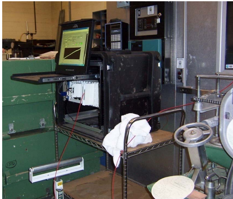
Figure 5: LVDT Data Collector
