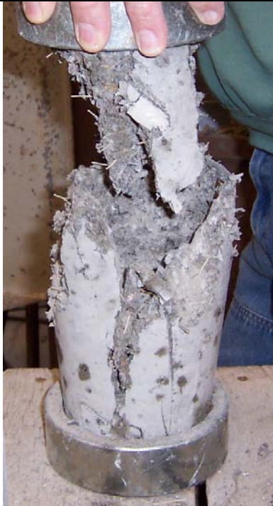
Figure 9: Cone Shear Failure
