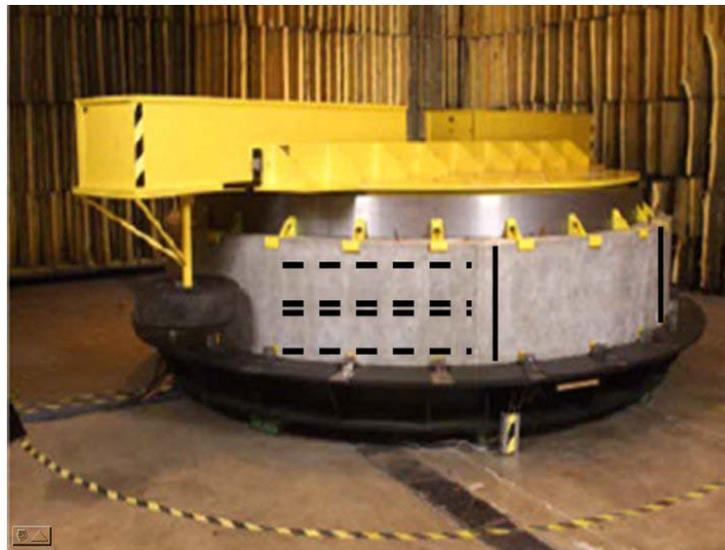
*Figure 2.2. Top Track Purdue laboratory testing wheel and diamond grinder.*
