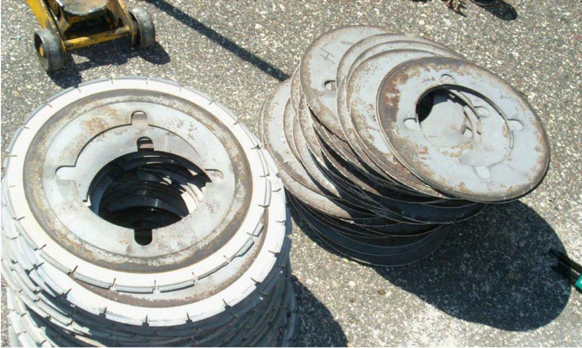
*Figure 2.4. Grinding head and spacers.*
