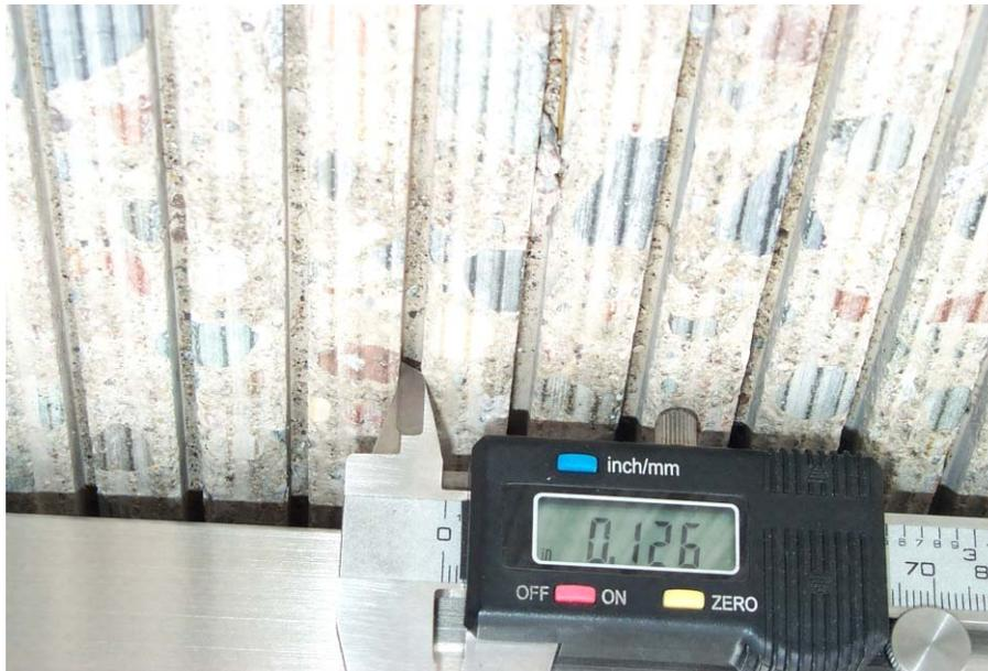
Figure 4.11. Ultimate grind groove width measurement.
