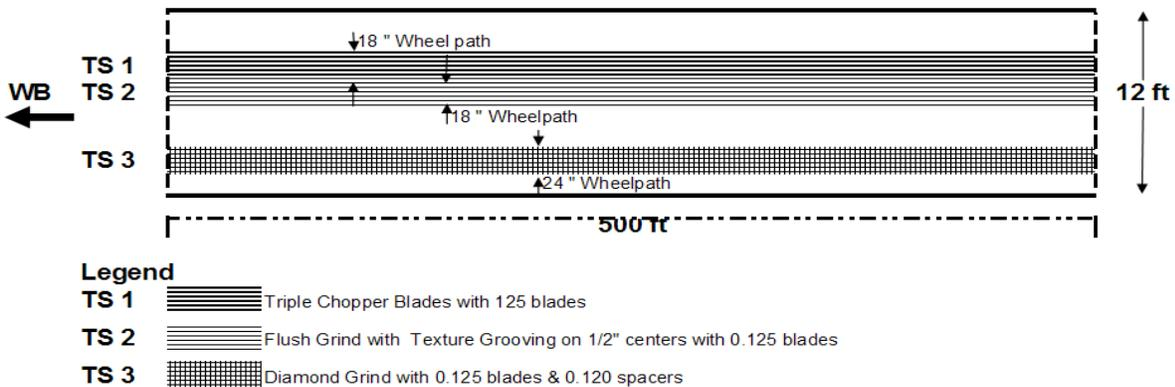
Figure 2.3. Diamond grinding test section layout on Cell 37.
