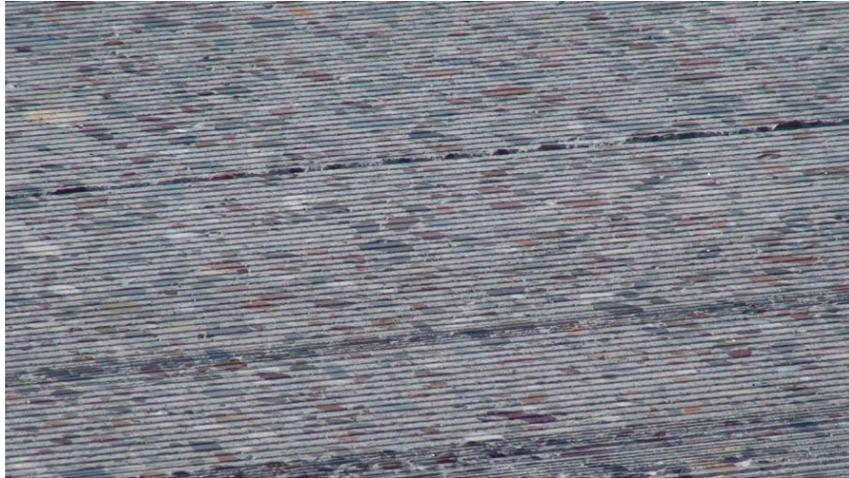
*Figure 4.6. Innovative grind with skid marks after friction testing.*
