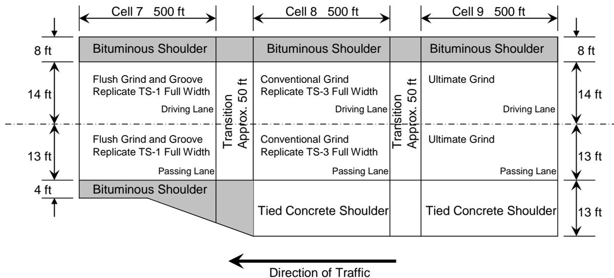
*Figure 4.1. Layout of grinding activities – Cells 7, 8, and 9.*
