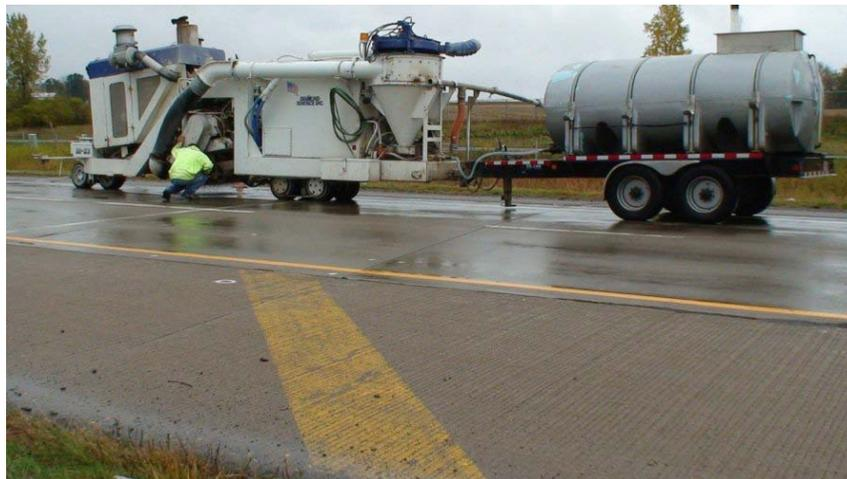
*Figure 4.2. DSI diamond grinding equipment.*
