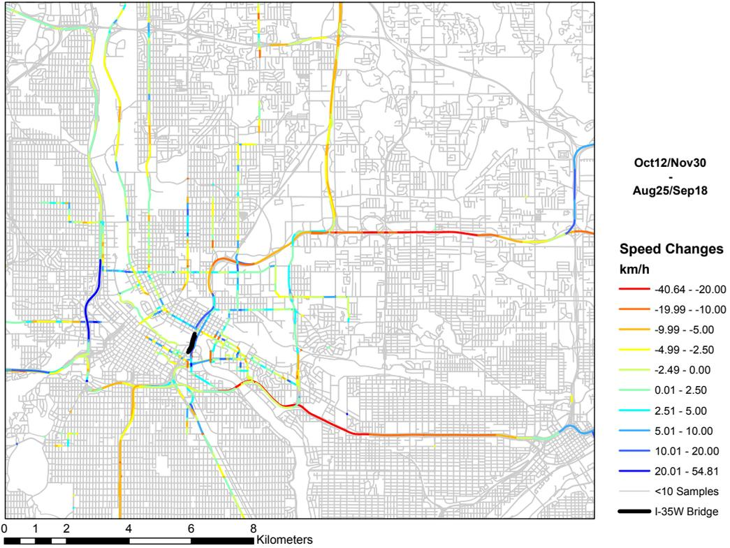
**Figure 7.2:** Speed changes during morning peak periods after the fourth through lane on I-94 Bridge was removed
