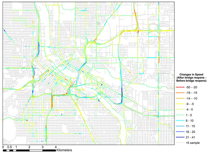
Figure 3.4: Comparison of travel speed before and after the replacement I-35W Bridge opened
